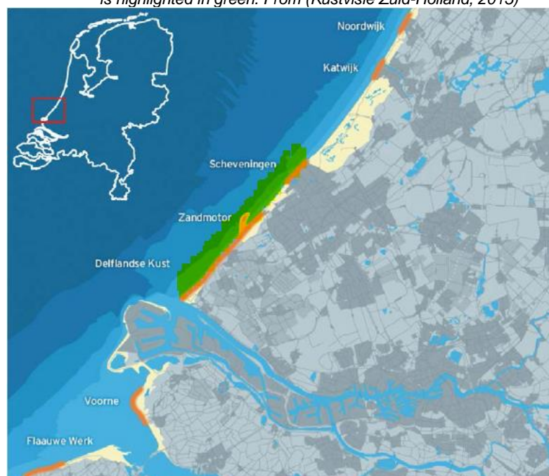
Figure 2.8 Location of the Sand Motor in the Delfland coast. The area between Hook of Holland and Scheveningen is highlighted in green. From (Kustvisie Zuid-Holland, 2015)
