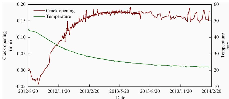
Fig. 13. The opening of fracture  $L_1$  measured by KM5-1 in tunnel #5.
