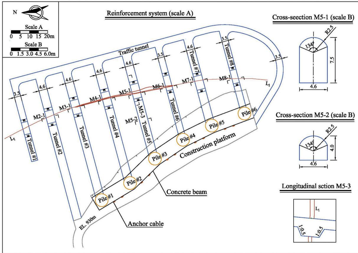
Fig. 5. Schematic diagram of the reinforcement system at EL. 930 m (Unit: m).
