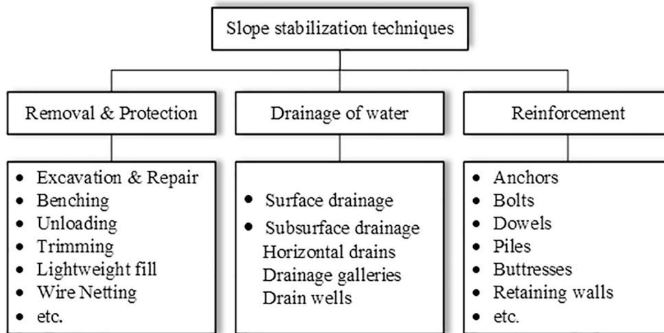
Fig. 1. Categories of slope stabilization techniques.
