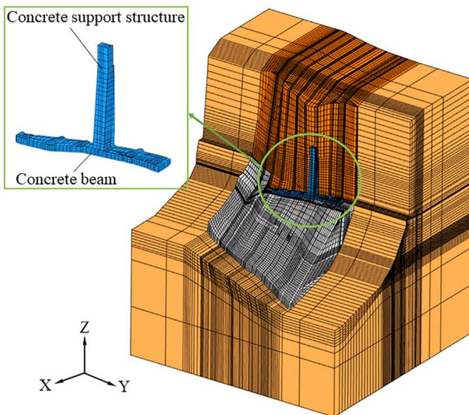
Fig. 6. Finite element mesh of the 3D model.
