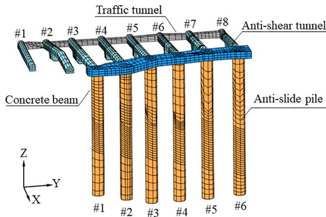
Fig. 8. Schematic representation of the finite element mesh model of the anti-shear tunnels and the anti-slide piles.
