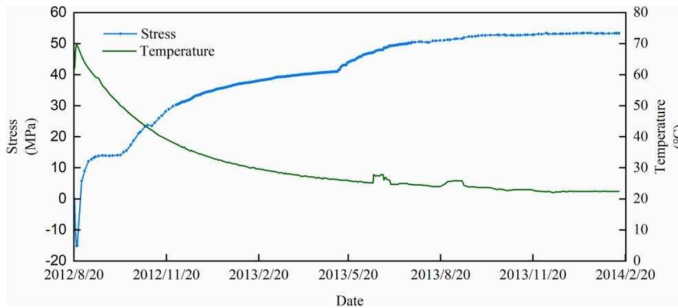
Fig. 12. The stirrup stress measured by RM5-14 in tunnel #5.
