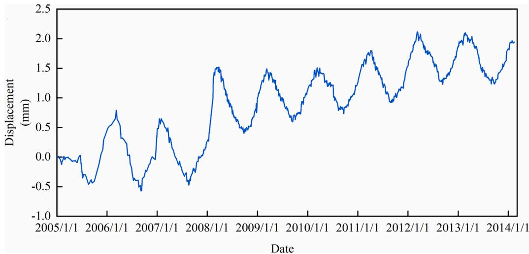
Fig. 10. The measured displacement of MDr2-4-2 at the top of the slope.
