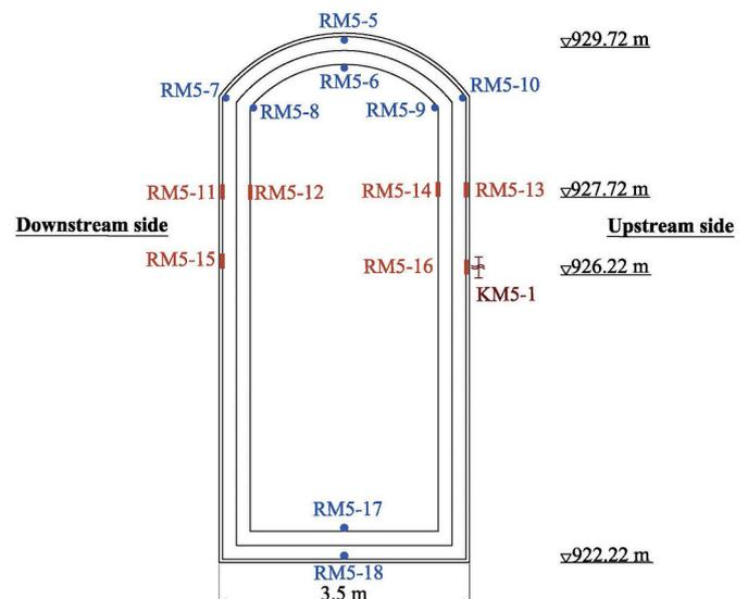
Fig. 11. The arrangement of stress meters and joint meters in tunnel #5 (the cross-section M5-1).
