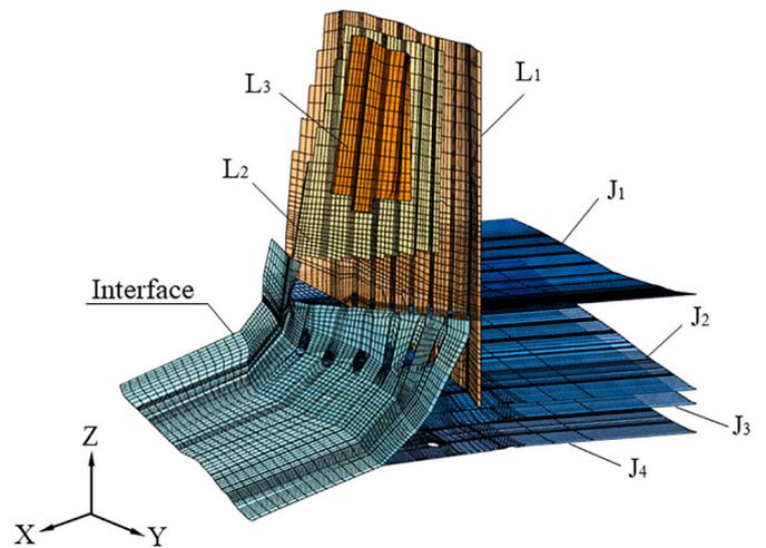
Fig. 7. Finite element mesh of the weak structural planes (Fractures  $L_1$ – $L_3$ , Intercalations  $J_1$ – $J_4$ , and the Interface).
