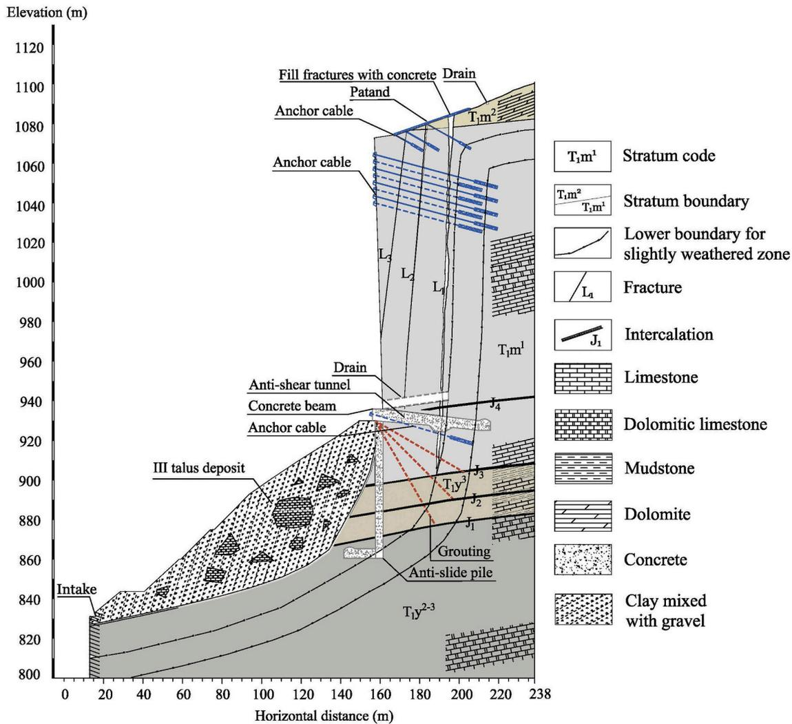
Fig. 4. Geological section of the reinforced Dr2 slope.
