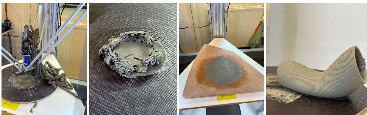
Figure 94, 95, 96, 97 accordingly: (Left) Material explosion. (Middle left) Printing failure. (Middle right) Adhesion strategy. (Right) Collided test. Own work.
