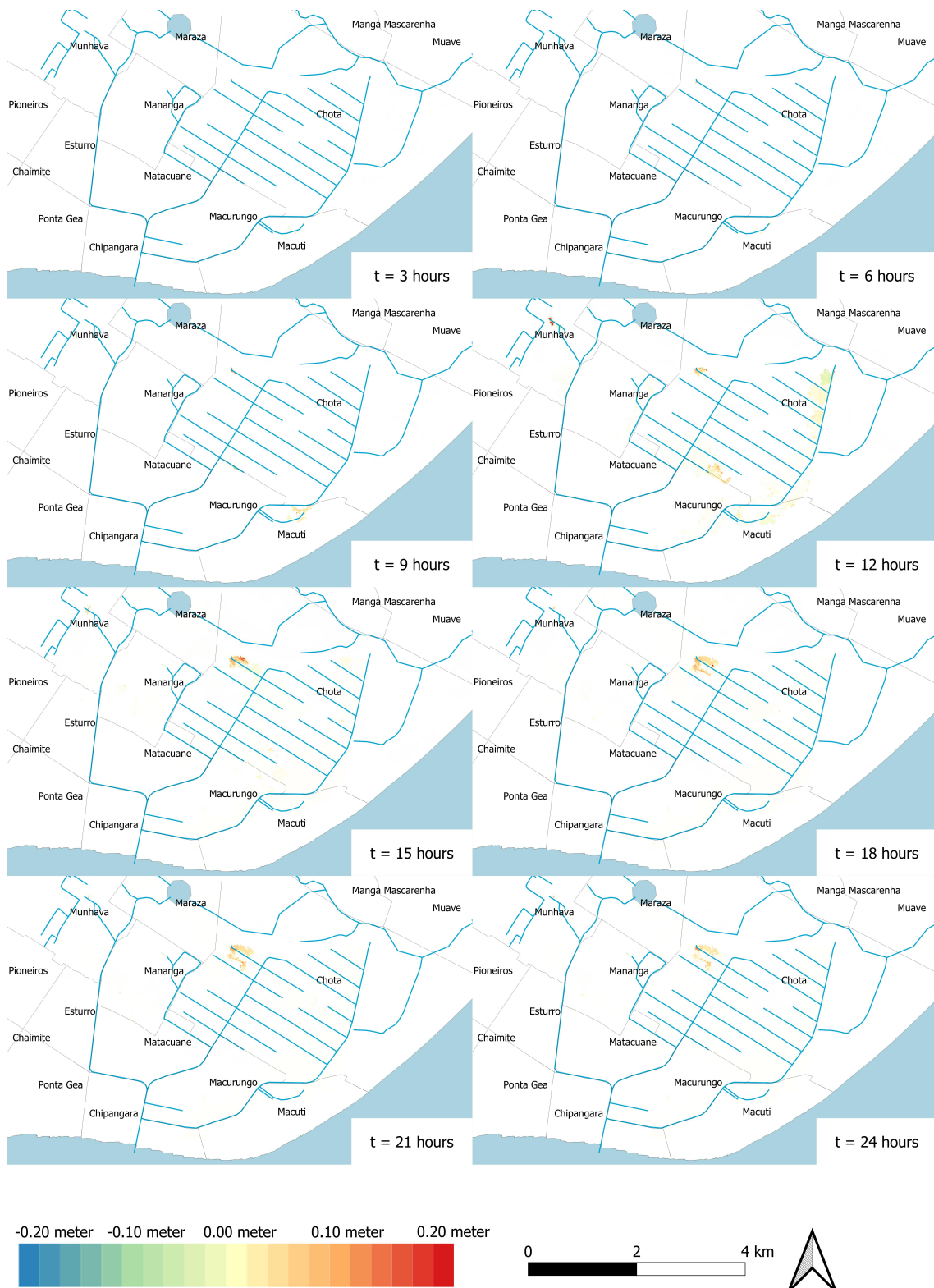
Figure F.10: Inundation depth increases in scenario 6: impact of blockage of the connections under precipitation event occurring once per 10 years
