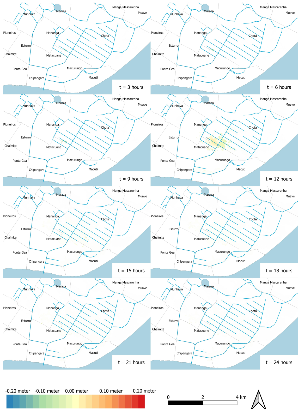
Figure F.9: Inundation depth increases in scenario 5: impact of waste in the Palmeiras outlet under precipitation event occurring once per 10 years
