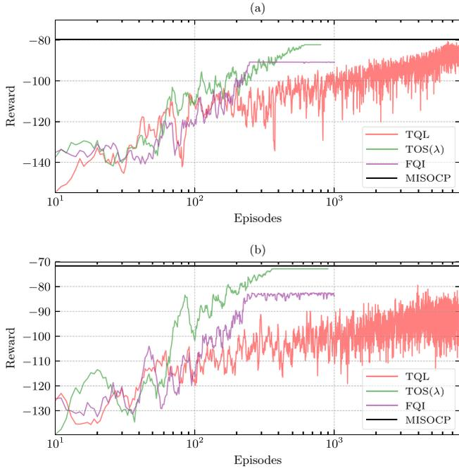
Fig. 5. Comparison of RL techniques learning curves for one day of operation. In this case, CESS has an EC = 500 [kWh]. Two different cases of SOC at the beginning of the day. (a) Case with SOC = 0 (b) Case with SOC = 0.5.
