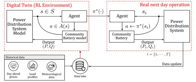
Fig. 1. RL agent learns to control a CESS under a digital twin network grid simulator, which uses actual historical data and current topology status of the grid. The learned policy  $\pi^*(\cdot)$  is deployed in real life for the next-day operation.
