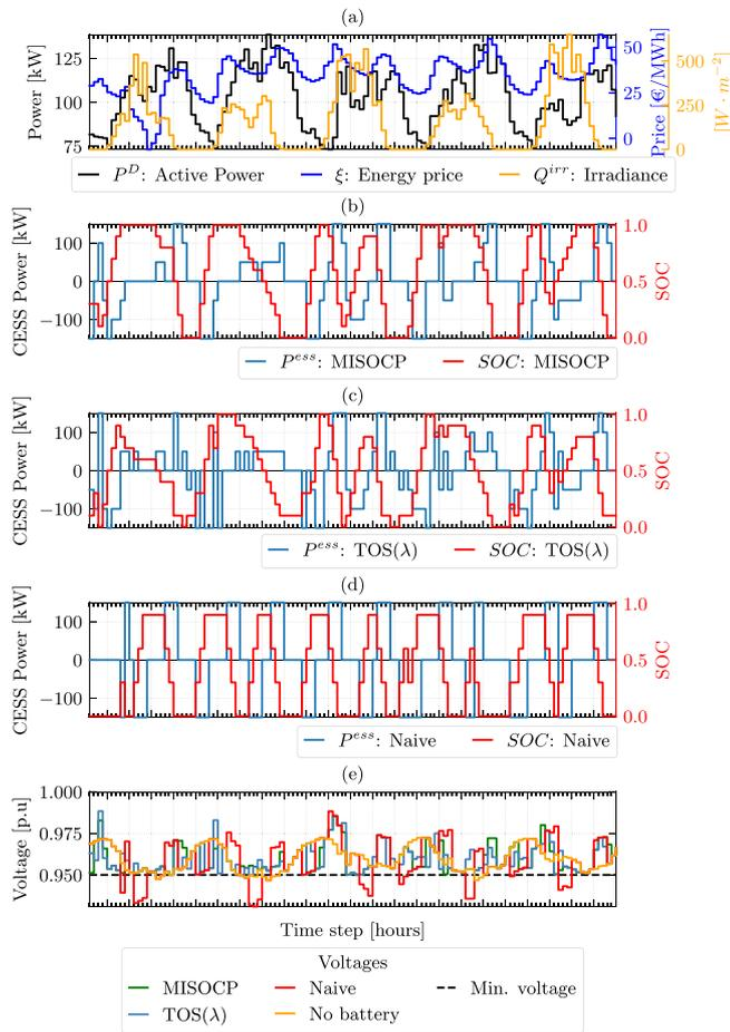
**Fig. 8.** CESS operation for a week with different methods. (a) Load consumption, solar irradiance, and energy prices at POC. CESS active power set points and SOC for: (b) MISOCP-Oracle, (c) TOS( $\lambda$ ), and (d) Naive charging policy. Subplot (e) show the voltages for the different solutions at POC.
