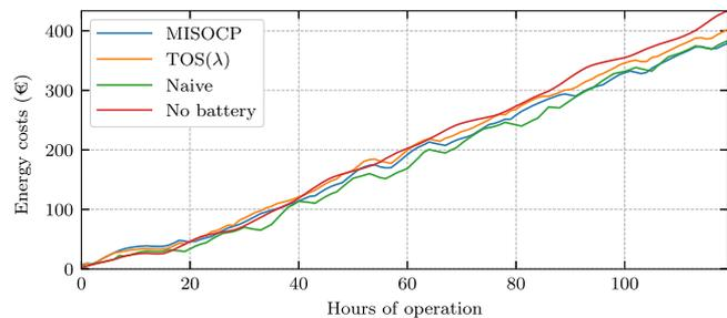
**Fig. 9.** Cumulative costs for a CESS of  $EC = 500$  [kWh] operating for a week with different controller methods.
