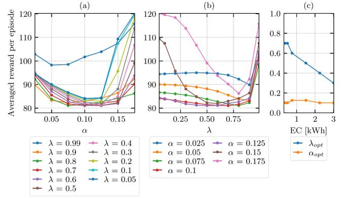
Fig. 6. Parameter sweep for Algorithm 1 for each combination of  $\alpha$  and  $\lambda$  shown in Table 1. Results reported are the mean averaged reward for the first 1000 episodes for 50 independent runs. (a) Parameter sweep viewed as function of learning rate  $\alpha$ . (b) Same parameter sweep viewed as function of decay rate  $\lambda$ . (c) Optimal  $\alpha$  and  $\lambda$  values for repeated sweeps as function of the battery size.
