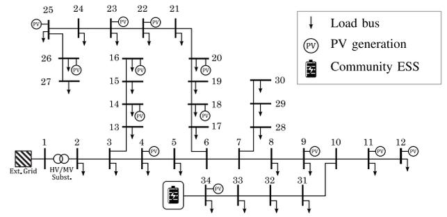
Fig. 4. Modified IEEE-34 Node bus test system with distributed PV generation. CESS placed in the longest feeder path as it is the worst-case scenario for grid's undervoltage problem.
