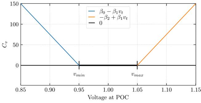
Fig. 2. Example plot of the Voltage penalty  $C_v$ , with parameters  $\beta_0 = 1425$ ,  $\beta_1 = 1500$ ,  $\beta_2 = 1575$ ,  $v_{min} = 0.95$  and  $v_{max} = 1.05$ . Values of voltage magnitudes outside technical limits at POC results in additional costs for the agent.
