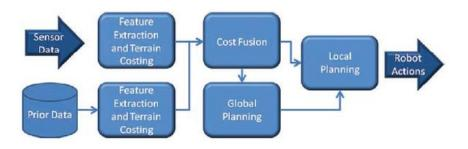
Figure 11 A high-level block diagram of the Crusher Autonomy system (Silver, Bagnell, & Stentz, 2010)
