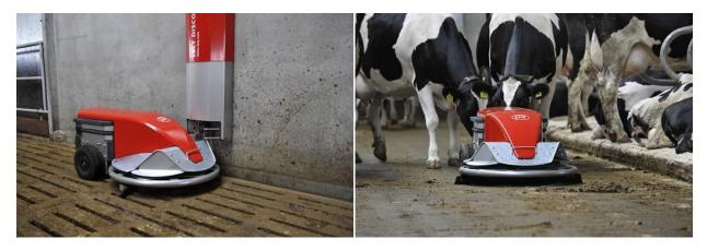
Figure 1 Lely Discovery Mobile Barn Cleaner (a) on the charger (b) cleaning
