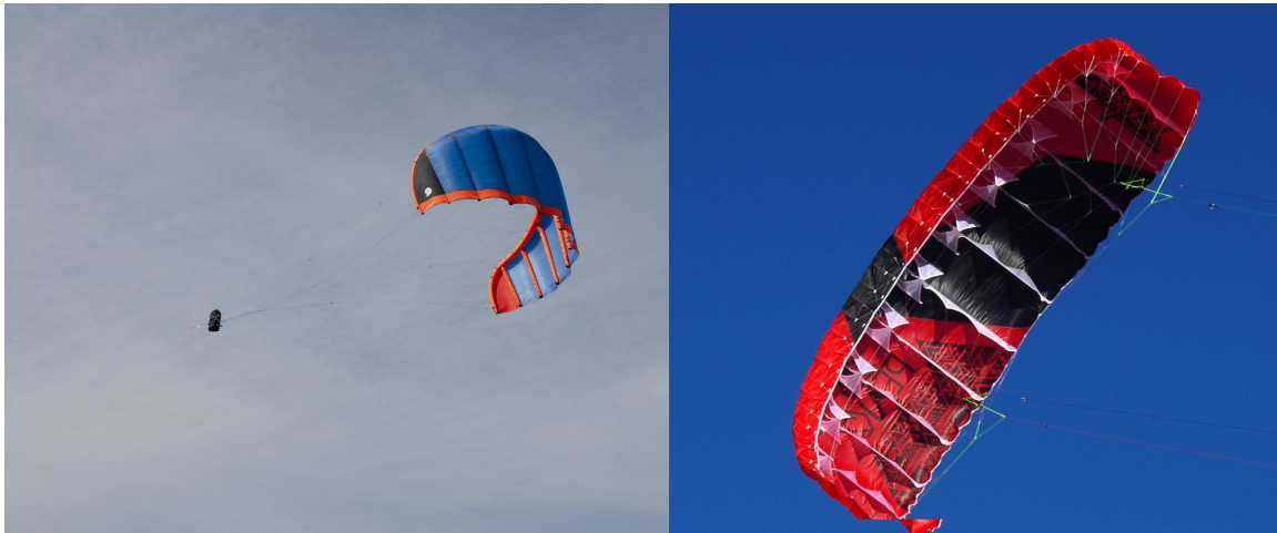
Figure 1.3: LEI kite from Kitepower (left) and Peak 2 Single Skin kite from Flysurfer (right) [31]
