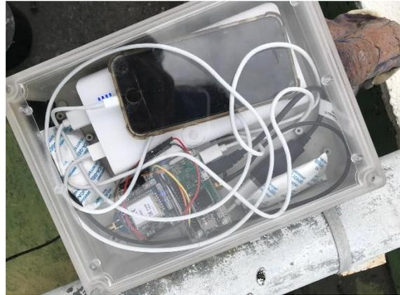
Picture 2: 'Base station' receiver, on top of Rayong Area Revenue -building in Rayong.
