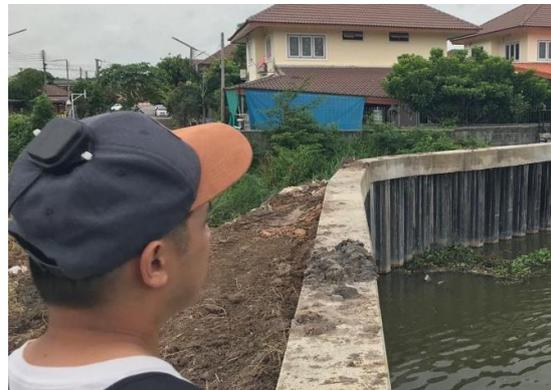
Picture 4: 'Rover' antenna for GNSS receiver, on top a cap to survey floodwall level while walking.
