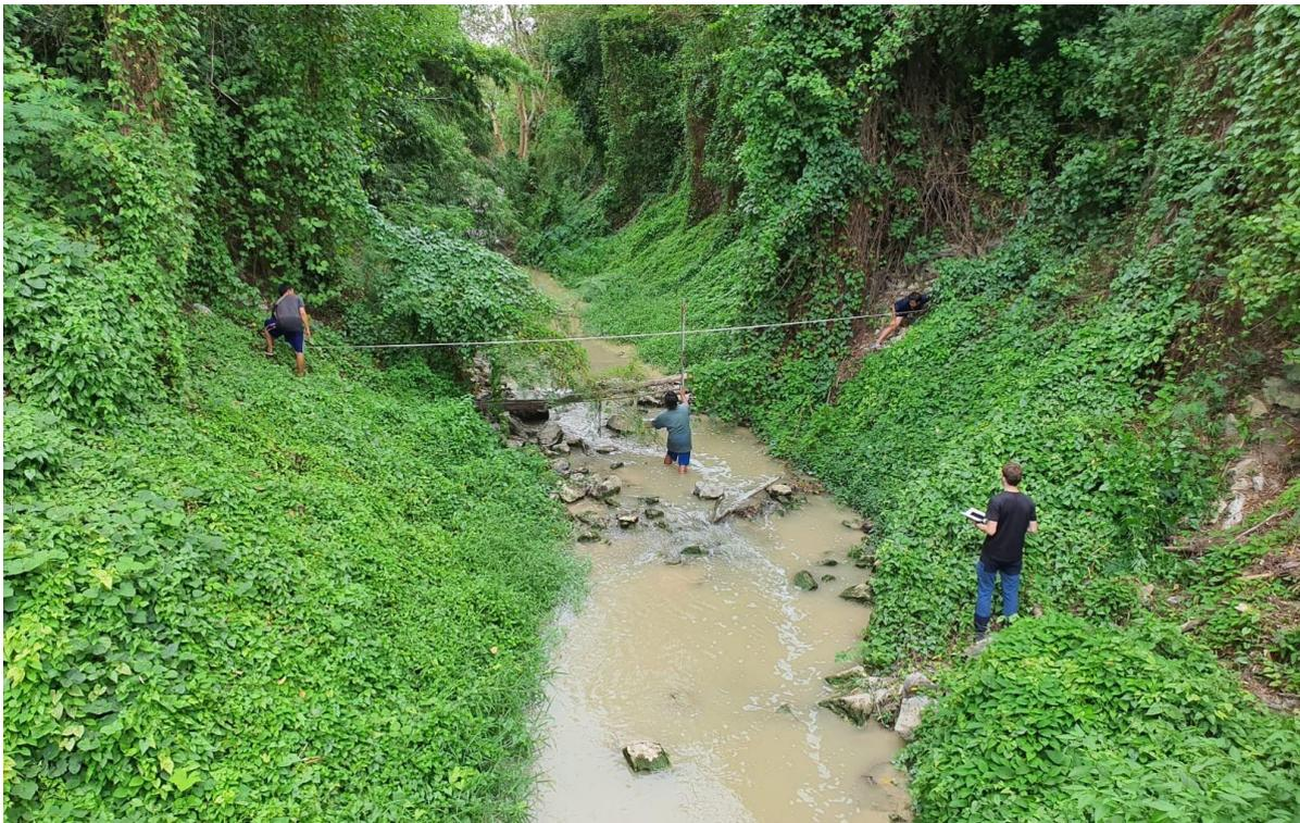
Picture 11: Bathymetry survey, picture was taken while the dry part of the cross-section was surveyed by measuring the width (y-axis) of the cross-section at every meter above water level.
