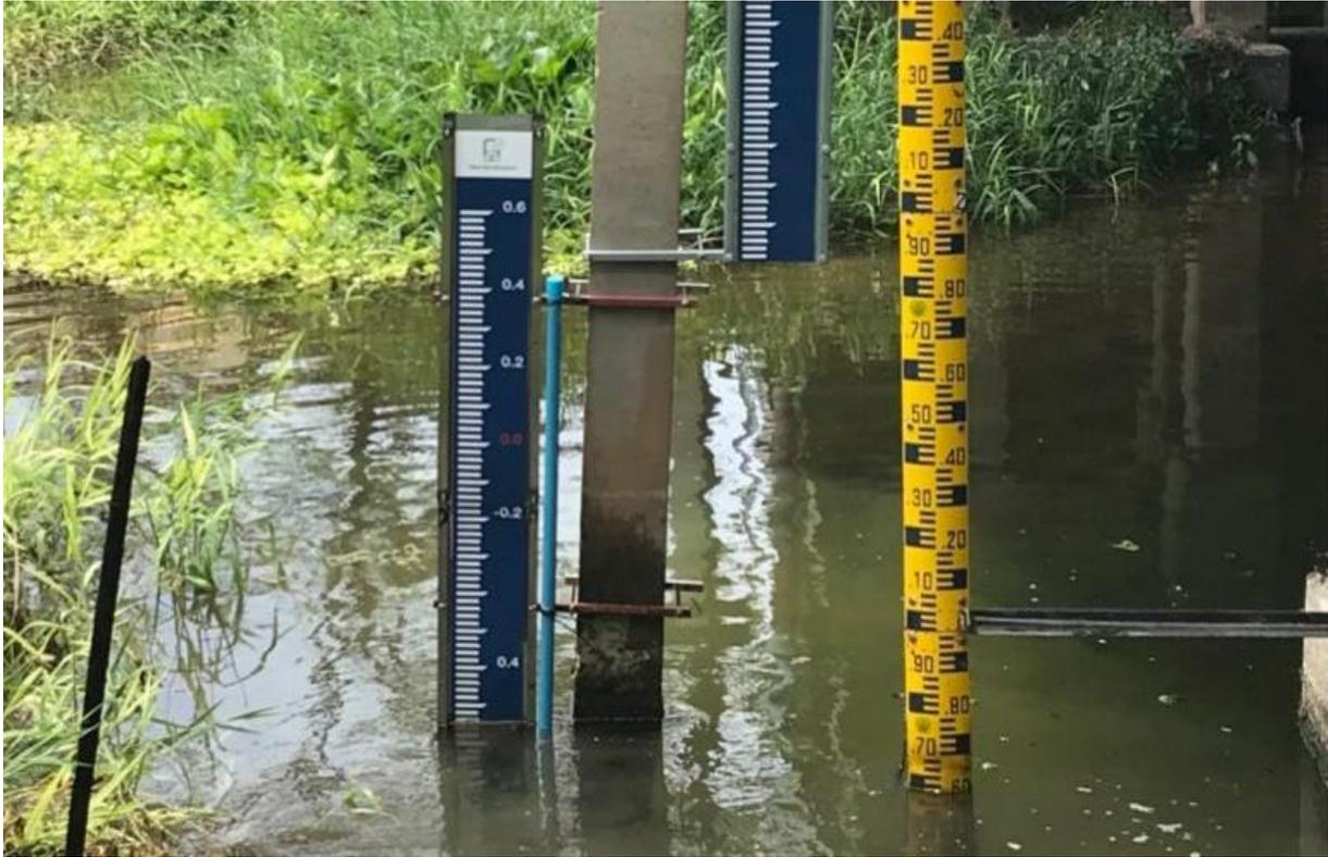
Picture 7: Water level survey at gauging station Z.38 with Mobile Water Management (blue staff gauge), Diver (inside blue PVC monitoring tube), and the original staff gauge from the RID (yellow staff gauge).
