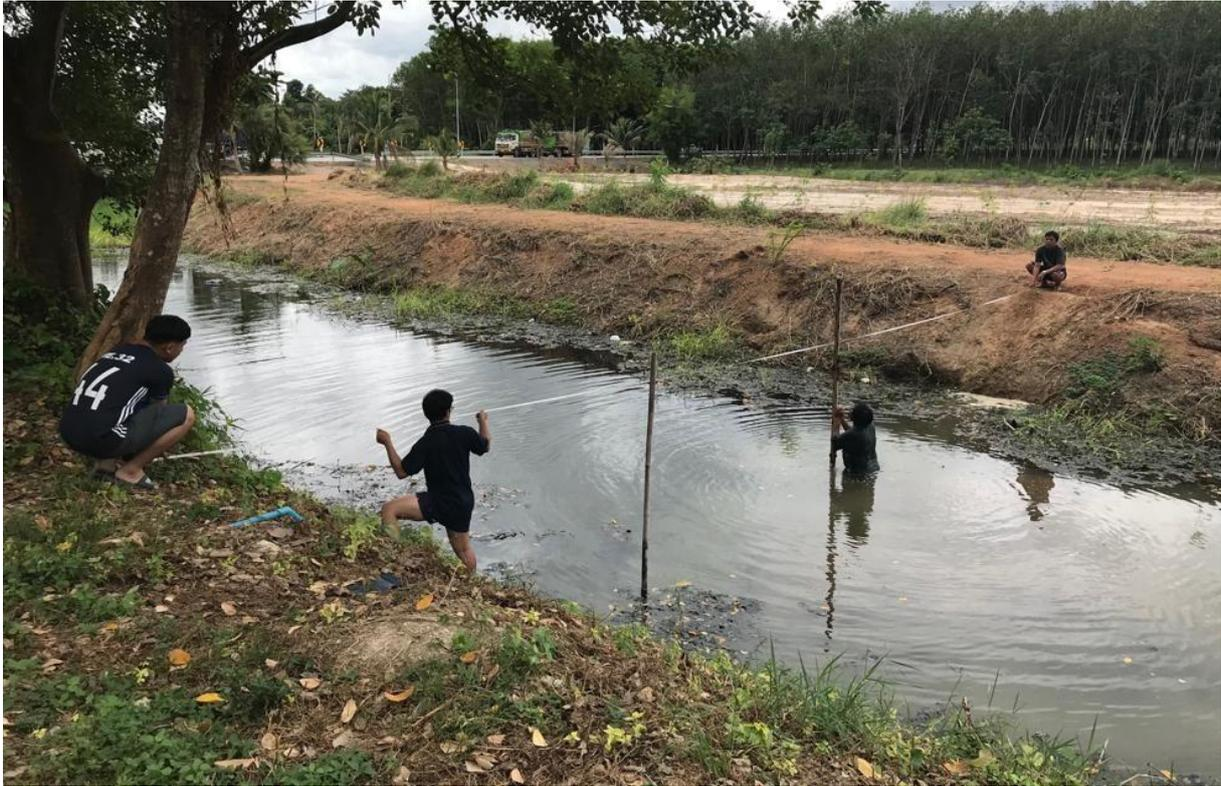
Picture 10: Bathymetry survey, picture was taken while the wet part of the cross-section was surveyed by measuring depth every 1 m over the y-axis of the cross-section.
