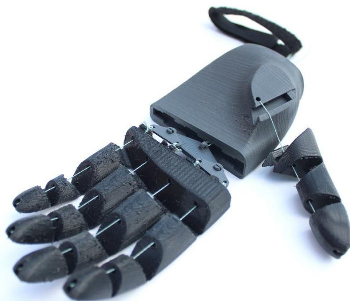
Figure 13: FR Hand partially disassembled. Assembly or disassembly doesn't require fasteners or tools
