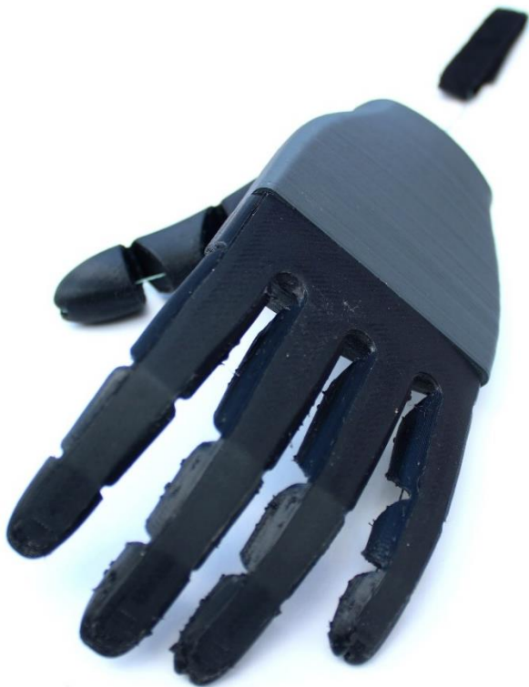
Figure 11: The FR Hand. The black parts are 3D printed in a flexible material, the grey parts are printed in rigid PLA plastic.
