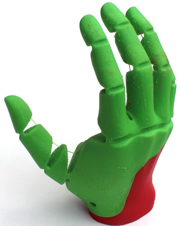
Figure 9: A prototype made using an existing adult 3D hand model, modified to use living hinges and to be 3D printed in two parts. The green part is made out of NinjaFlex flexible material, the red part is printed in rigid PLA plastic. Braided Teflon-coated fishing wire is used for the actuation strings.
