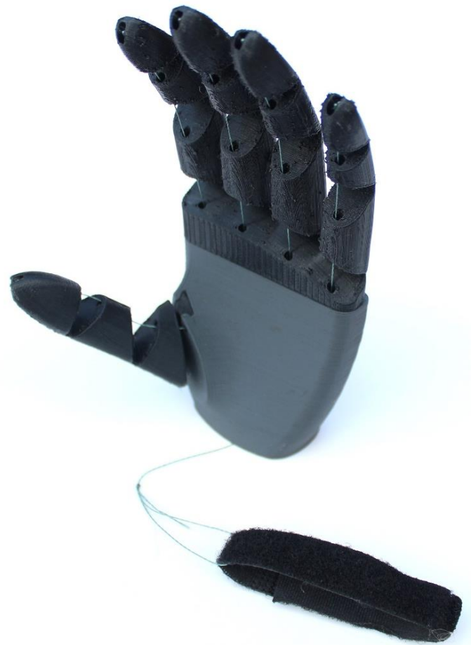
Figure 10: FR Hand, pulling the string actuates the fingers and thumb
