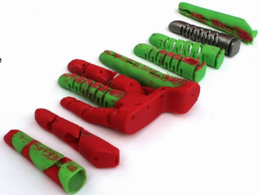
Figure 8: A selection of 3D printed hinge design prototypes. Every design was printed in place, no assembly was required. The green material is NinjaFlex flexible material, the red material is rigid PLA plastic. The red residues left on some of the green parts are left over support material. One variation of the "coil spring" finger was printed in steel.
