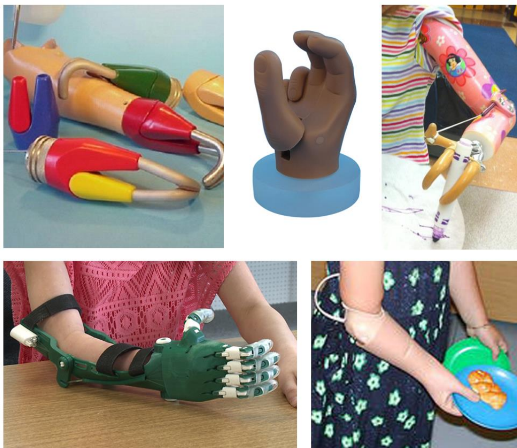
Figure 1: Selection of prosthetic arms specifically designed for children. From the top left, clockwise: WILMER appealing prehensor, TRS Child Lite Touch Hand, conventional split hook, 3D printed wrist actuated prosthetic hand, myoelectric arm prosthesis. For image credits see Appendix A.1.
