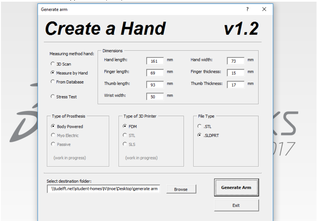
Figure 20: The Graphical User Interface (GUI) that allows a user to generate a custom sized prosthetic hand
