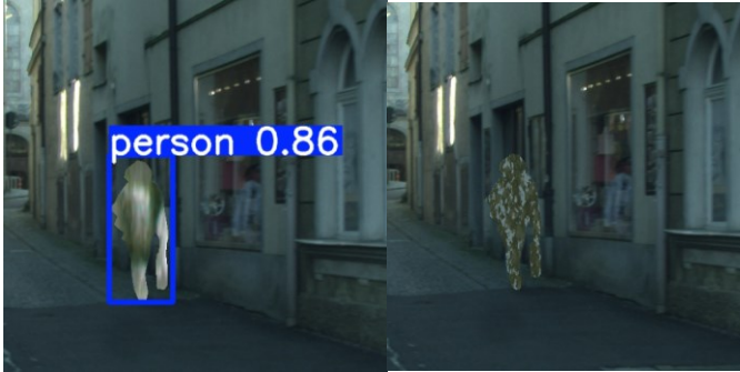
Figure 5. Visualization of detection performance by a computer vision model with camouflage applied to a person's silhouette. The images show the comparison between CamoGAN (left) and CamoX (right), which the computer vision model completely fails to recognize. Reproduced from Nguyen et al. (2025).
