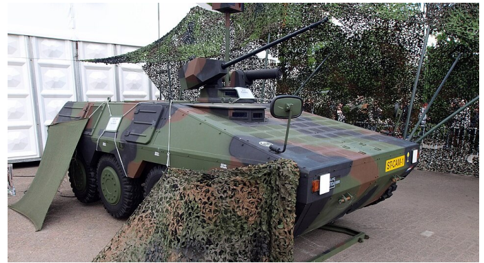
Figure 1. Photograph of STANDCAM, (STANdard Decoy for CAMouflage Materials) a standardized, non-classified, armored vehicle-shaped target developed by Germany's Wehrtechnische Dienststelle 52 to measure and test the effectiveness of camouflage materials. Photograph by van Beem (2012).
