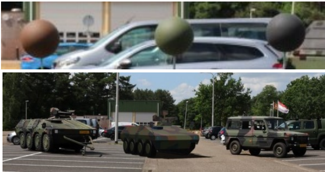
Figure 3. Top: three painted spheres in the same colors as the camouflage pattern, used for lighting information in the hybrid (material capture) method. Bottom: A hybrid scene generated using the material capture method. The middle vehicle is the virtual object. Reproduced from van der Sanden et al. (2023).
