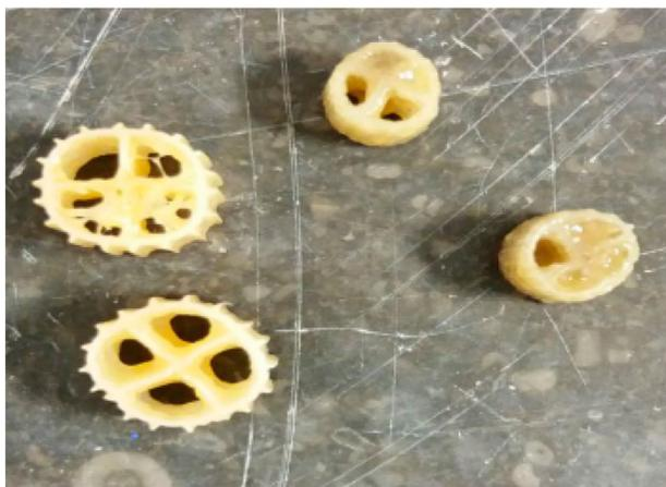
**Figure 8.** Kaldnes K1 micro carriers still almost full of biomass after PS feeding and Kaldnes K1 carriers which have very thin layer of biofilm after PS feeding.
