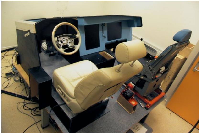
Figure 4.7: Fixed-Based Simulator at HMI lab TU Delft [33]
