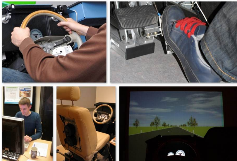
Figure 7.4: Fixed based driving simulation (HMI lab), different elements [33]
