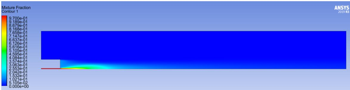
**Figure 5-8:** Contour of mixture fraction for FGM model.
