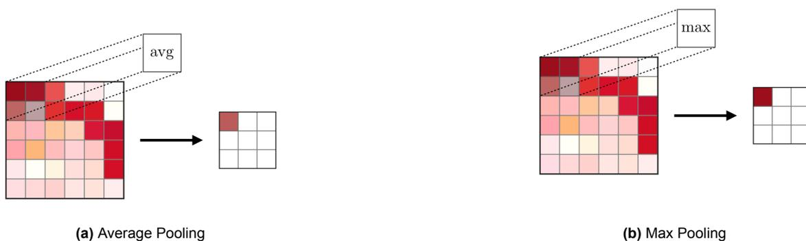
Figure 2.6: Types of Pooling
