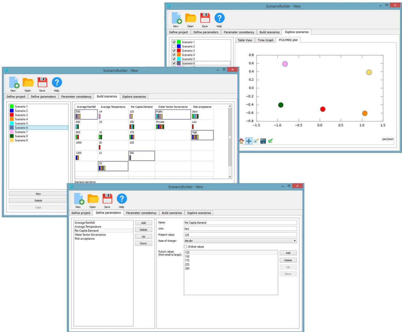
**Figure 8.** Screenshots of the Scenario Planner Tool. The user can compose scenarios based on a defined set of parameters, add values, and perform internal consistency checks. Once defined, a scenario is visualised. The user can then export the scenarios for use in UWOT.
