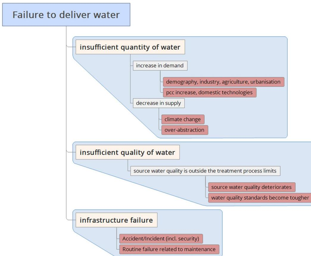
**Figure 2.** Different functional (quantity and quality) and structural (infrastructure) failure modes of water services for the water quantity objective.
