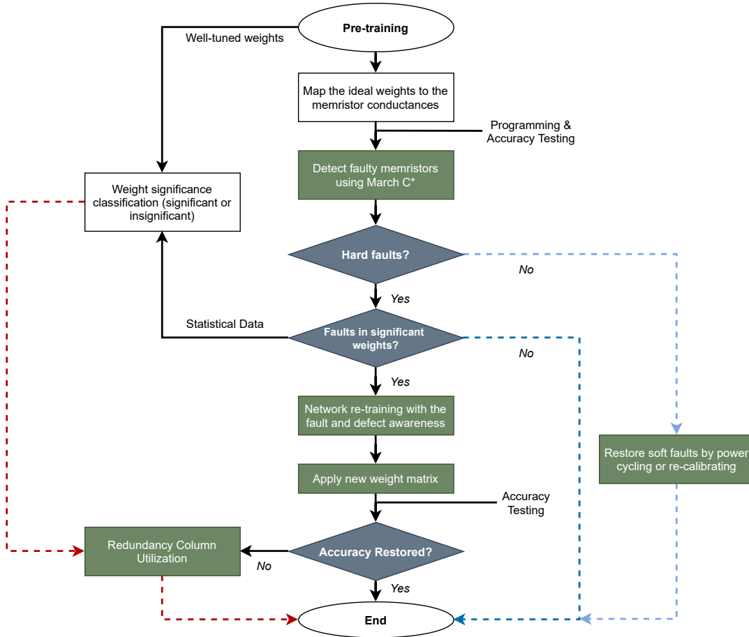
Figure 4.17: Schematic image of the proposed reliability scheme incorporating the novelty of both [103] and [79]. The process begins with a pre-trained and validated neural network, which is then mapped to hardware before being used to compute the neural network whilst maintaining accuracy. Filled elements in the flowchart describe activities during run time on the neuromorphic computing engine. Adapted from a diagram presented in [103].
