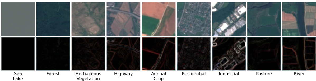
Figure 5.1: Example images of each of the land cover classes provided in the EuroSAT dataset, with RGB versions in the top row [99] and Prewitt-filtered versions in the bottom row [9].
