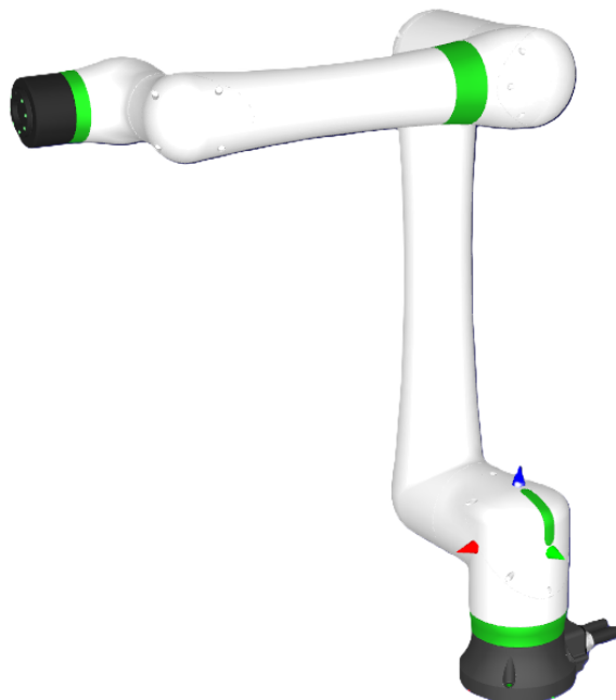
Figure 5.1: Reference of the origin of the robotic arm.
