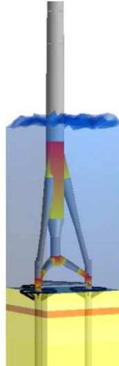
Figure 40 Fatigue damage of the main joints of the tripod support [23]
