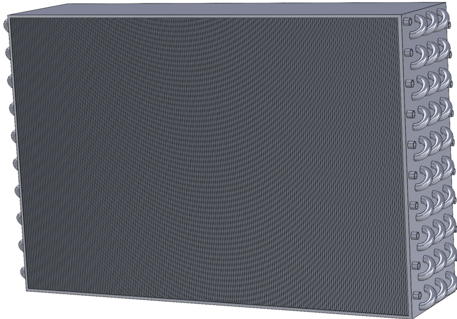
Figure 3.8: Illustration of the plate-finned tube heat exchanger design. Cold air flows through the face of the radiator. Liquid electrolyte is distributed across the tube rows; containing multiple tube passes.
