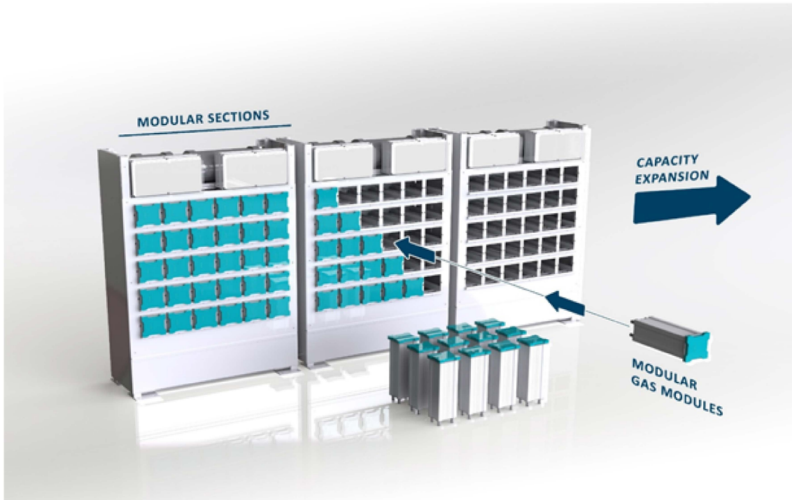
Figure 1.5: Illustration of the modular section in the XINTC system. Each section functions as a stand-alone unit, and allows for convenient system capacity alteration. Each section includes electrolyzer modules, heat exchangers, gas-liquid separators, and a flow panel.
