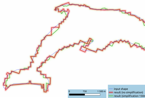
(b) GPS art results. Red - without simplification of the input, green - simplification threshold of 150 meters. Thin blue line is the original, non-simplified input.
