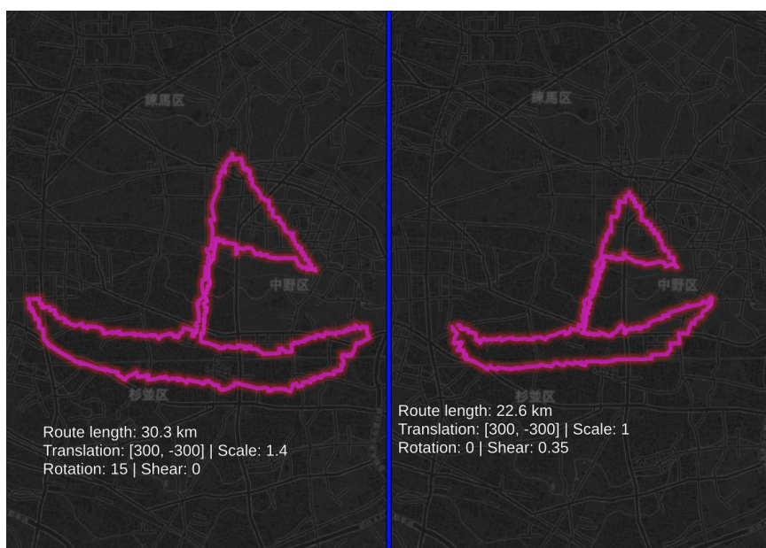
Figure 3.4: Example two GPS art route candidates for an input sailboat drawing. These particular candidates have different scale, rotation and shear
