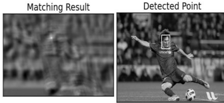
Figure 2.2: Example template matching solution to detect a person's face. Source: OpenCV tutorial
