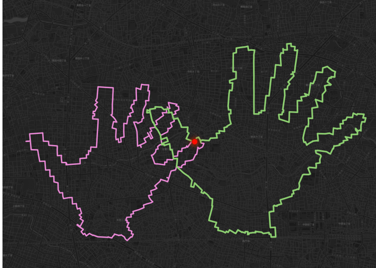
Figure 3.16: Example two distinct artistic route candidates which satisfy the constraint of a starting point (red marker)
