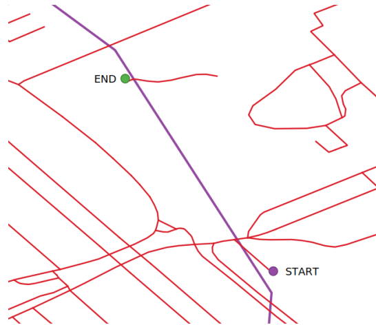
Figure 3.23: Example of a disconnected street segment (red) which causes a routing failure. The routing start and end node are labelled. The input shape segments are colored purple.
