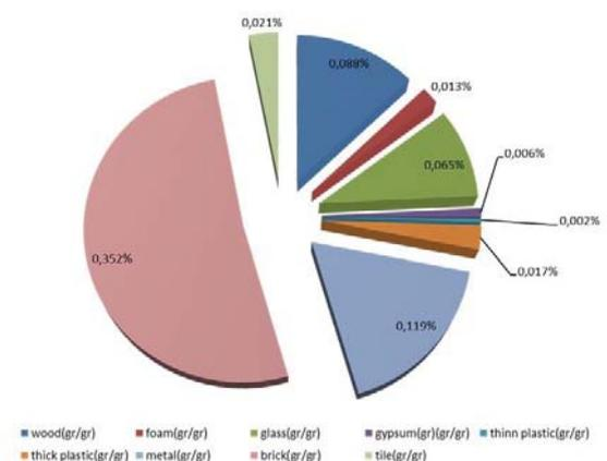
Figure 5: Constituents of the contaminants mixed with concrete.
