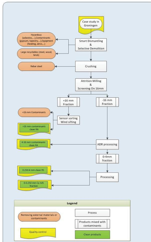
Figure 1: General layout of the C2CA technology showing different steps for contaminants removal. Two developing sensors (HSI and LIBS) are being developed for the quality control of the products.
