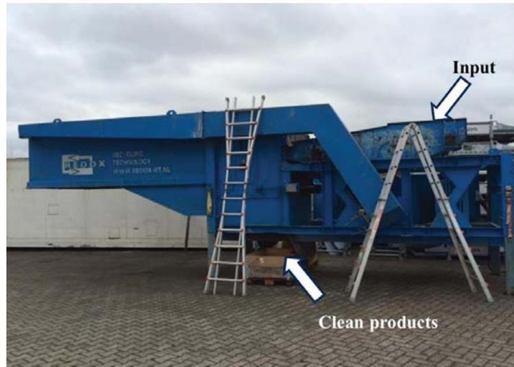
Figure 10: Wind sifting facility in REDOX.
