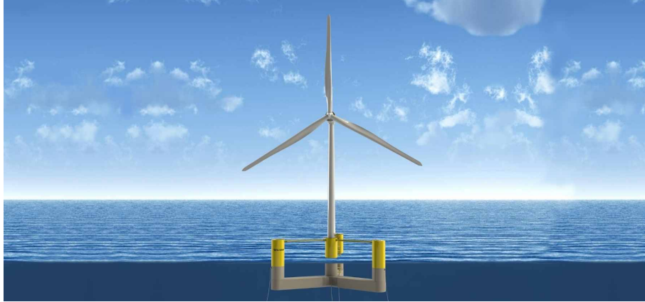
Figure 1.2: Rendering of the IEA 15 MW reference wind turbine mounted on the UMaine VoltturnUS-S semi-submersible floating platform [5], the reference system used throughout this thesis. Image: University of Maine Advanced Structures and Composites Center [6].
