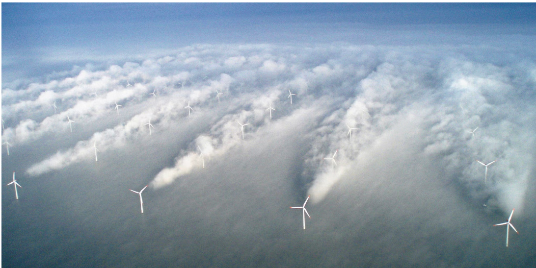
Figure 2.1: A light fog reveals the wake effect behind turbines at Vattenfall’s Horns Rev wind farm off Denmark. Photo: Vattenfall
