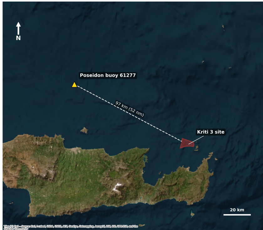
Figure 3.13: The Kreti 3 site (red polygon) north-east of Crete and the Poseidon E1M3A measurement buoy (WMO 61277, yellow triangle), located approximately 97 km (52 nm) to the north-west. Satellite basemap: Esri World Imagery.
