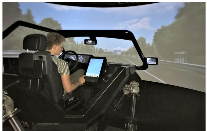
Fig. 1. The AS2 6DoF motion-based Cruden driving simulator with the setup used during the experiment.
