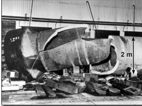
**Figure 1.1:** Pressure vessel failure during hydraulic test [1].
