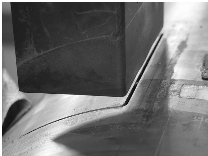
**Figure 7.5:** EDM cutting of the central window with the L-shaped electrode after having performed one of the two cuts required for the rectangular window.
