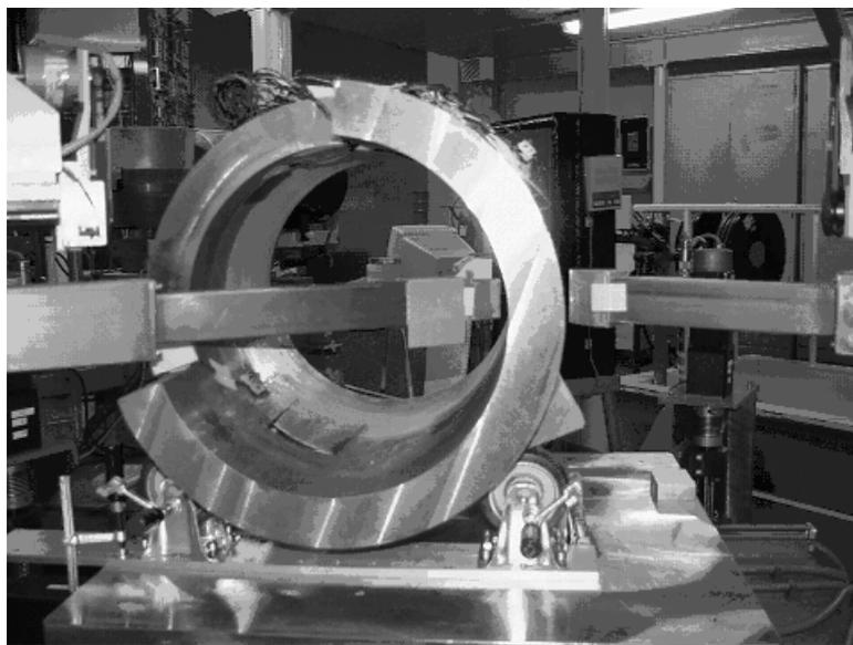
**Figure 7.18:** *Dissimilar metal weld component during the neutron diffraction measurements in the piping axial direction. Cf. Fig. 7.15.*
