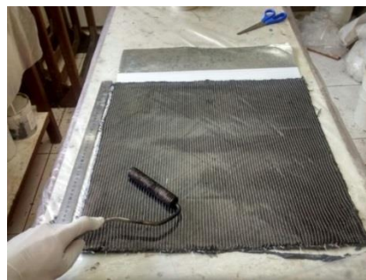
Fig. 1 Carbon fiber lamination process
