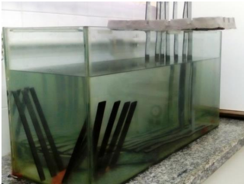
33 Fig. 3 Specimens in salt water tank
