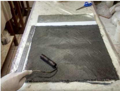
Fig. 1 Carbon fiber lamination process
