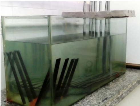
Fig. 3 Specimens in salt water tank
