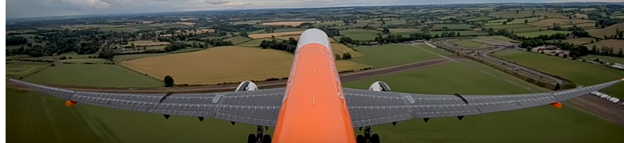
(b) Folding wingtips in horizontal position during cruise
