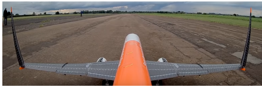
(a) Folding wingtips in vertical position during taxiing
