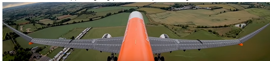
(c) Folding wingtips released for gust load alleviation
