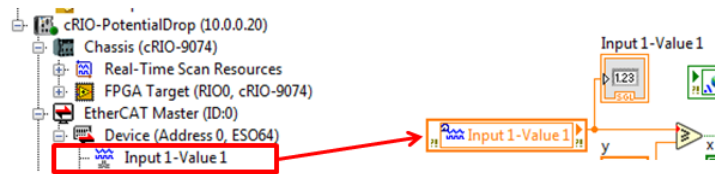
Figure A.16: Dragging I/O variables from the LabVIEW project to the block diagram
