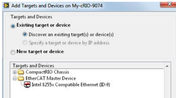
Figure A.12: Selecting the EtherCAT Master Port on the Real-Time Controller.
