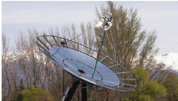
**Figure 1.2:** *Travelling wave thermoacoustic engine with using solar heat to produce electrical power made by Qnergy, Utah.*
