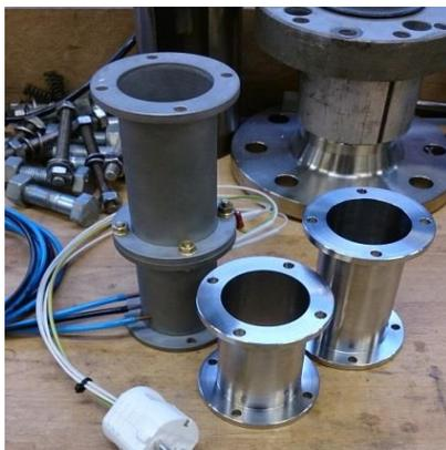
**Figure 3.4:** *Assembly of the second regenerator tube.*
