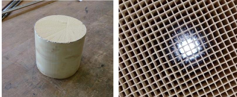
**Figure 3.1:** *Ceramic catalyst used as regenerator material.*
