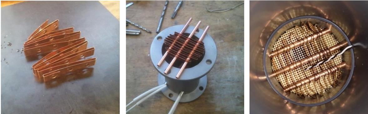
**Figure 3.6:** *Construction of the cold heat exchanger.*
