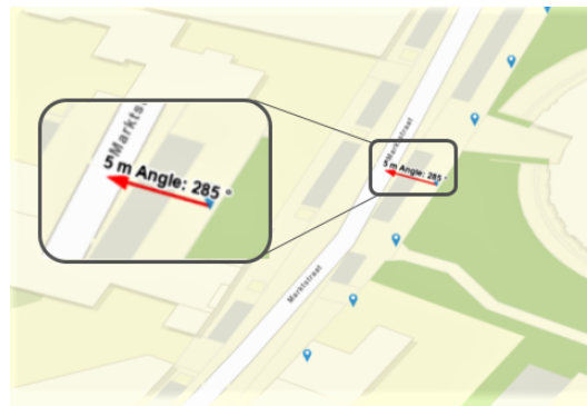
Figure 4.7: A visible GPS offset in the dynamic dataset in a residential area in Echt, The Netherlands.
