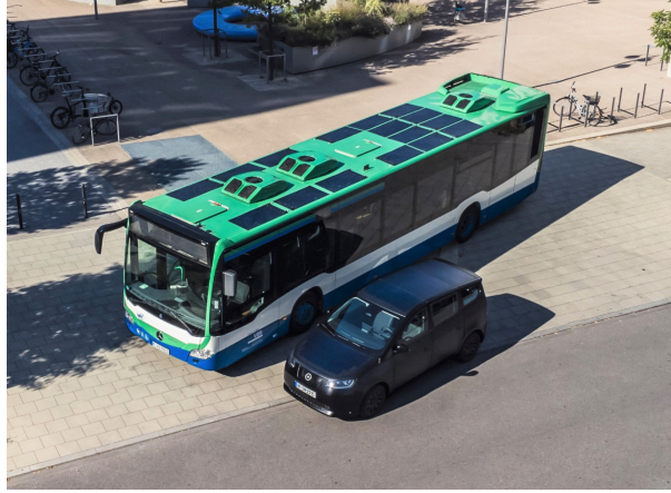
Figure 1.2: The two chosen vehicle categories differing in vehicle height, a passenger car and public transport bus with integrated PV, from Sono Motors [23].
