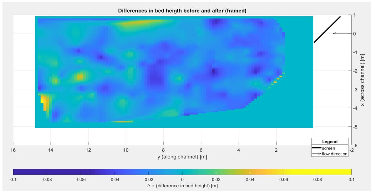
Figure 4.4: Plot of the differences between the bottom profile before and after, framed to get rid of outliers (run 8)
