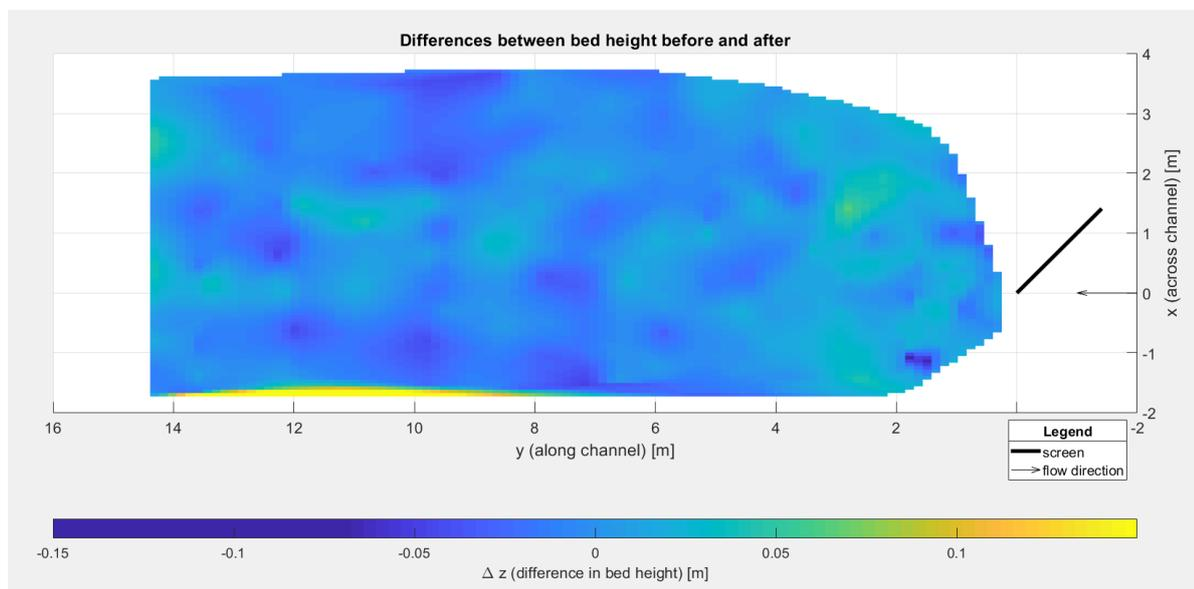
Figure B.13: Plot of the differences between the bottom profiles before and after (run 7)
