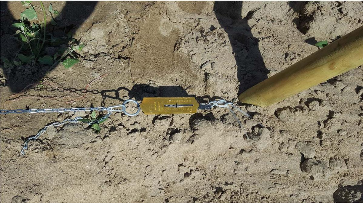
Figure D.9: Close-up of one of the used spring scales
