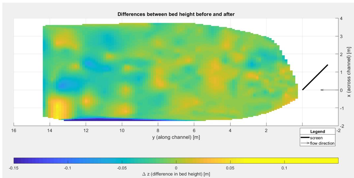
Figure B.11: Plot of the differences between the bottom profiles before and after (run 6)
