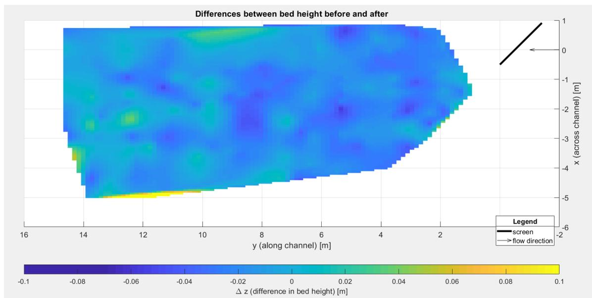
Figure B.15: Plot of the differences between the bottom profiles before and after (run 8)
