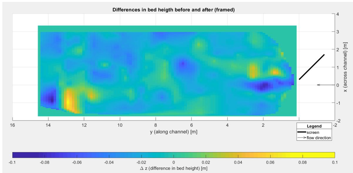
Figure 4.3: Plot of the differences between the bottom profile before and after, framed to get rid of outliers (run 5)
