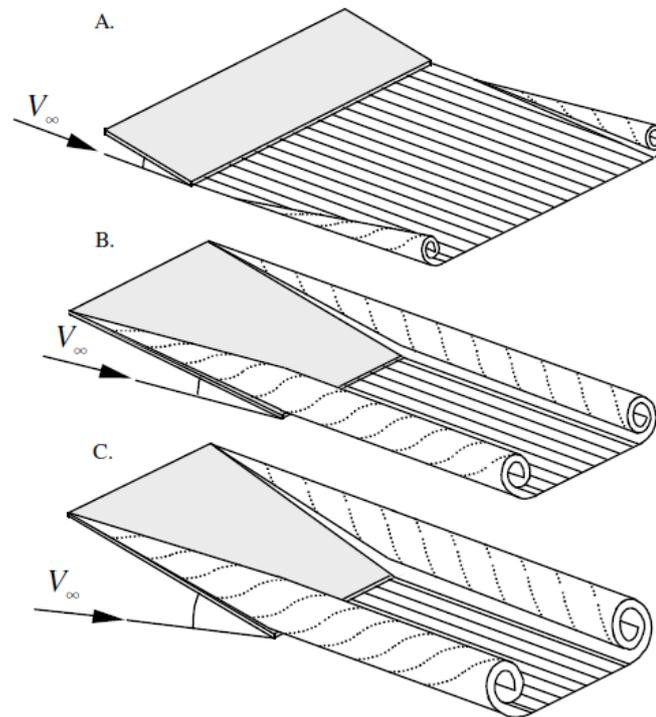
Figure 2.2: Vortex formation for high aspect ratio wings (A) and low aspect ratio wings (B,C) (Van Zwol, 2004)
