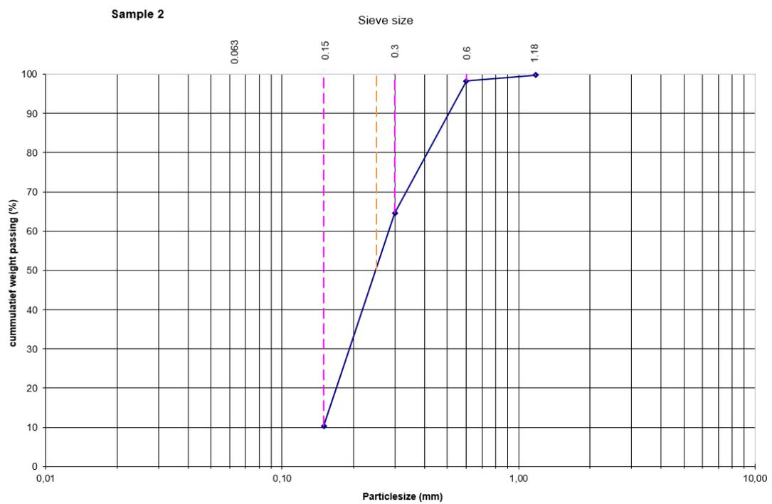
Figure A.2: Sieve curve for sediment sample 2. Indicated  $D_{50} = 0.25$  mm.
