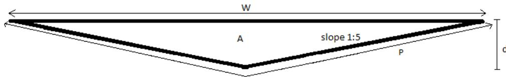
Figure 3.2: Simple representation of the cross profile of the Welsumerwaard channel, derived from Rademakers (2016).
