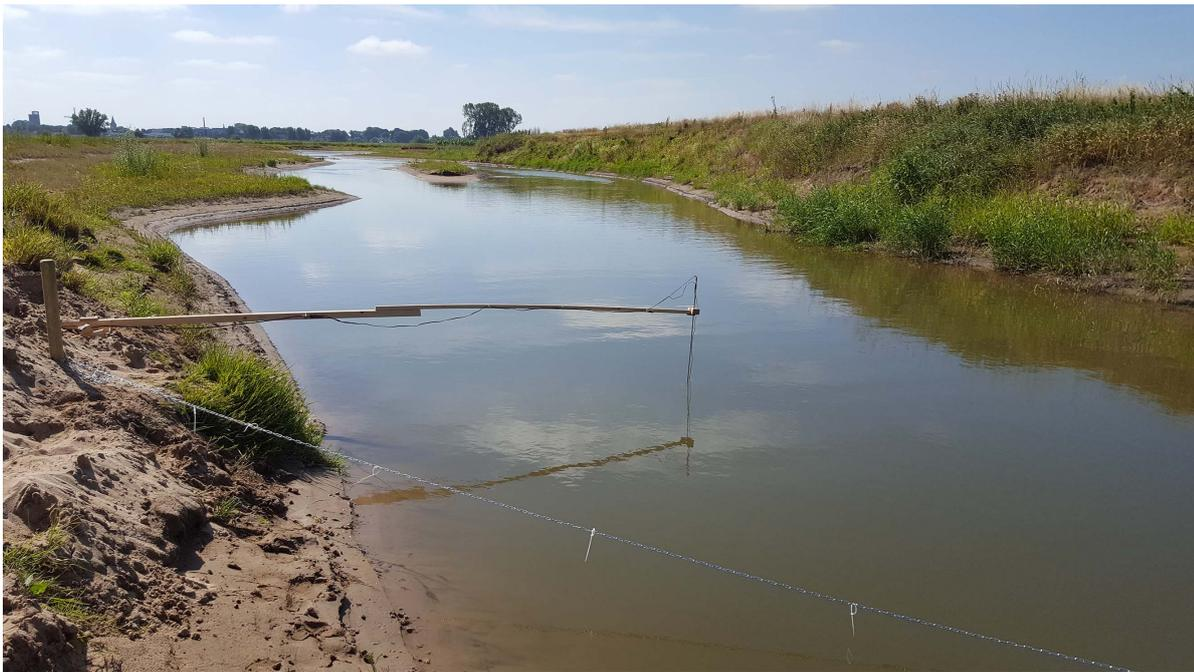
Figure D.4: Arm with current meter attached (below water surface)
