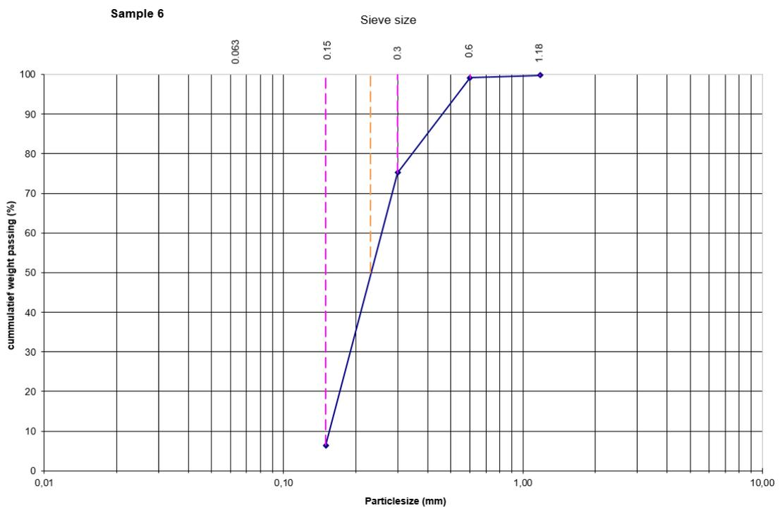
Figure A.6: Sieve curve for sediment sample 6. Indicated  $D_{50} = 0.23$  mm.
