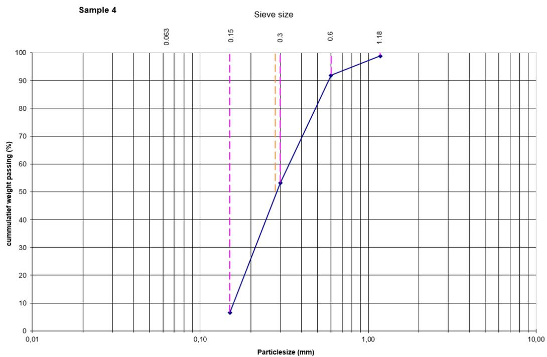
Figure A.4: Sieve curve for sediment sample 4. Indicated  $D_{50} = 0.28$  mm.
