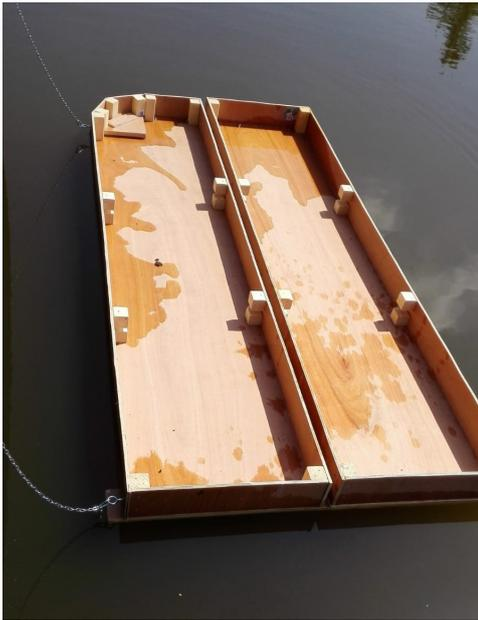
Figure D.11: First test in water: leaking observed
