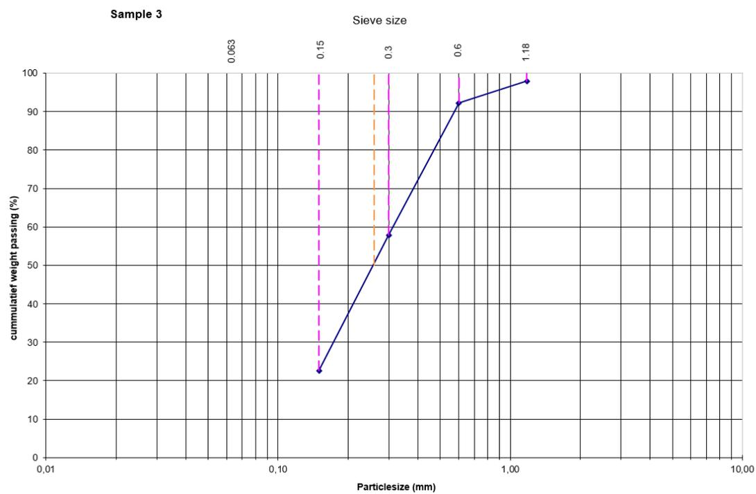
Figure A.3: Sieve curve for sediment sample 3. Indicated  $D_{50} = 0.26$  mm.
