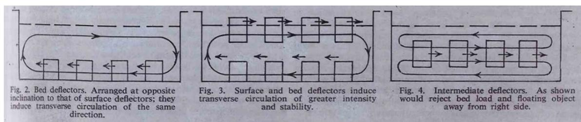
Figure 2.1: Formation of transverse flow by screens (Batalin, 1961)
