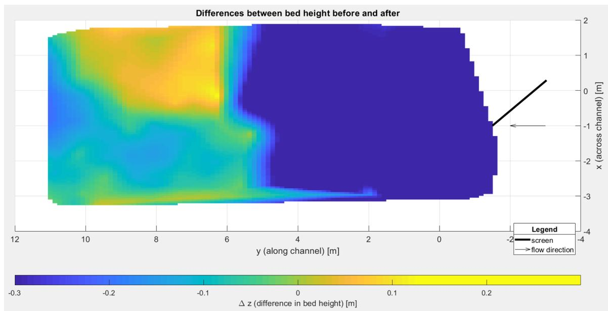
Figure B.4: Plot of the differences between the bottom profiles before and after (run 4)
