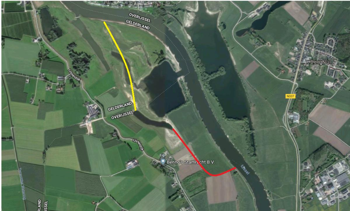
Figure 3.3: Satellite image of the Welsumerwaard. The channel has been constructed along the red line, the yellow line and the existing water bodies. The red line indicates the part that is considered for the experiments (Google Maps). The total length of the side channel is about 2 km.
