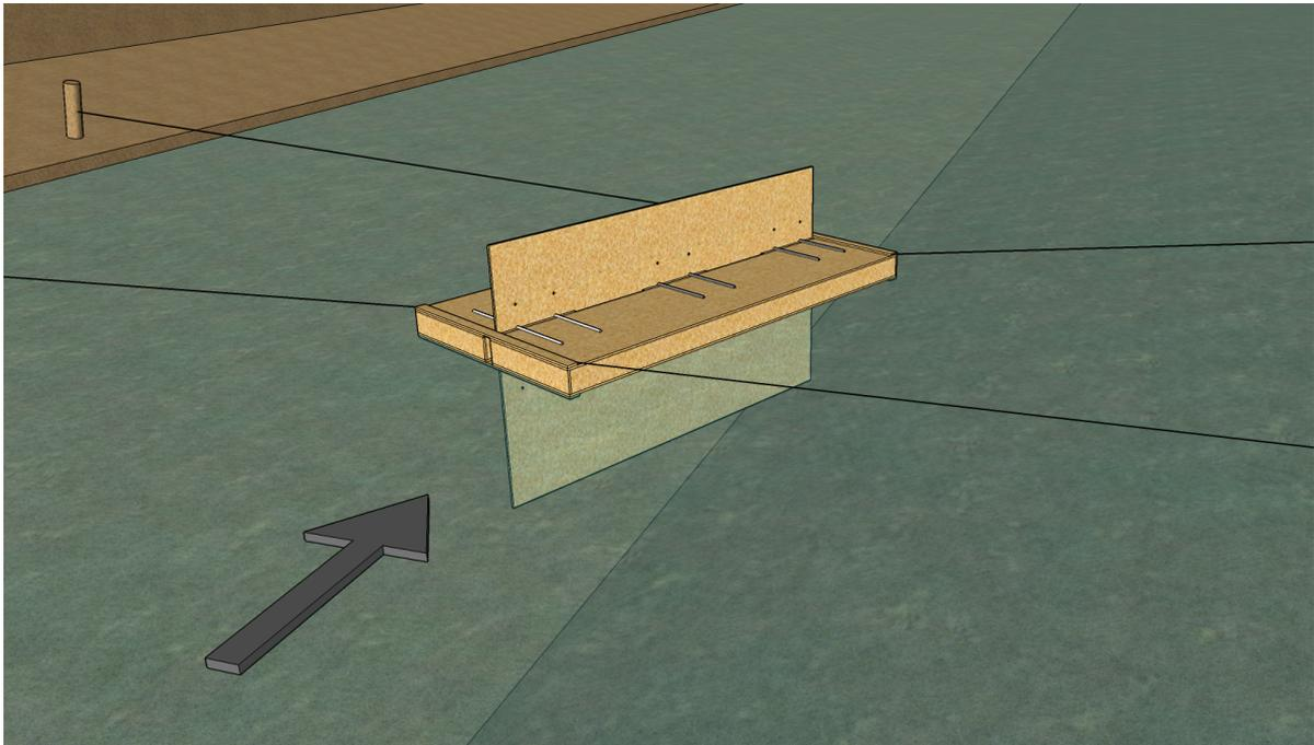
Figure 3.6: Screen with floating boxes. Arrow indicates flow direction. Water depth = 1.0 m; Penetration = 70%; Angle of attack = 25 °
