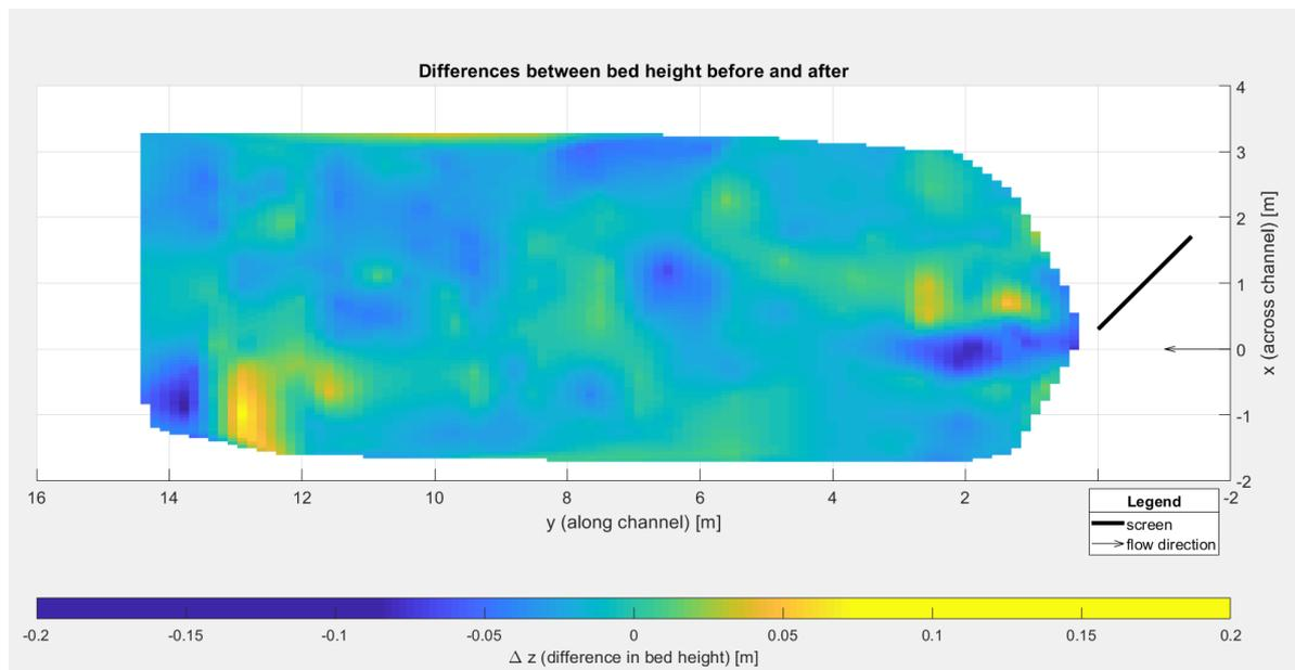
Figure B.7: Plot of the differences between the bottom profiles before and after (run 5)
