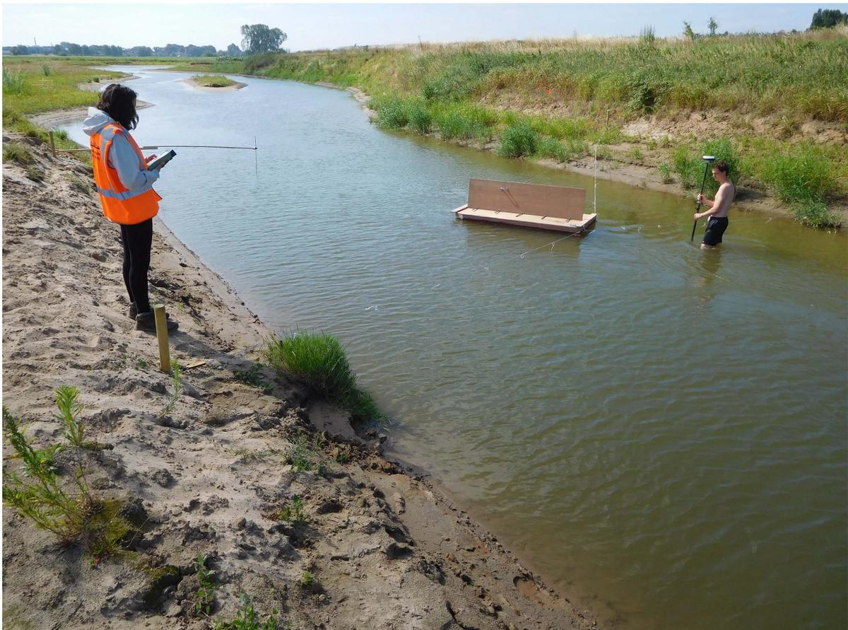
Figure D.8: Measuring the bottom profile using a GPS
