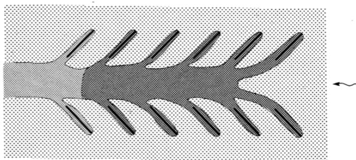
Figure 4.5: One of the setups of Filarski (1966). Legend: dark: erosion > 20%; intermediate: erosion < 20%; light: sedimentation.
