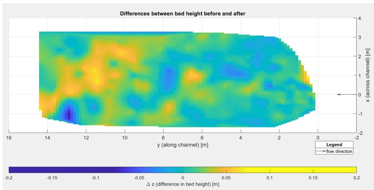
Figure B.9: Plot of the differences between the bottom profiles before and after (period 5-6)
