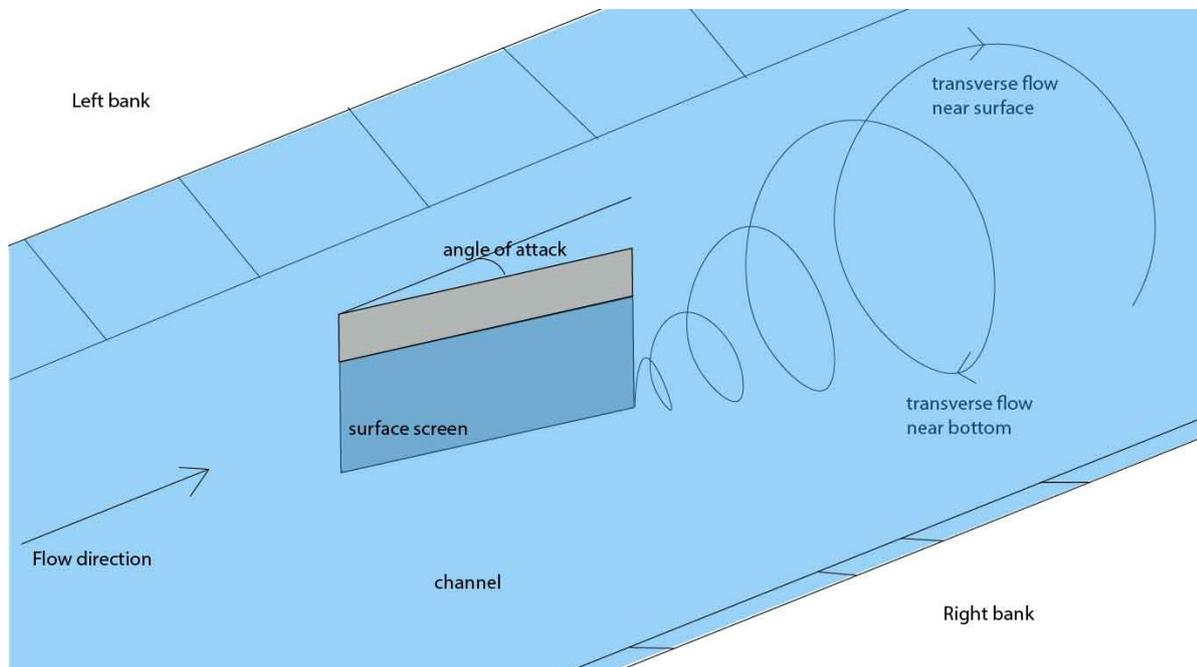
Figure 2.3: Simplified picture of vortex formation by a surface screen
