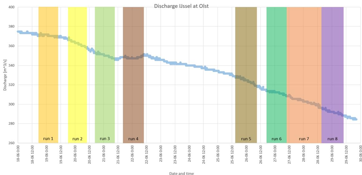
Figure 4.1: Discharge in the IJssel at Olst in m<sup>3</sup>/s. (Runs are indicated with the shaded areas)
