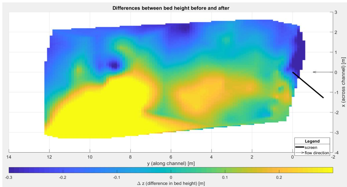
Figure B.3: Plot of the differences between the bottom profiles before and after (run 3)
