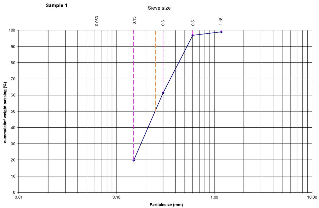
Figure A.1: Sieve curve for sediment sample 1. Indicated  $D_{50} = 0.25$  mm.
