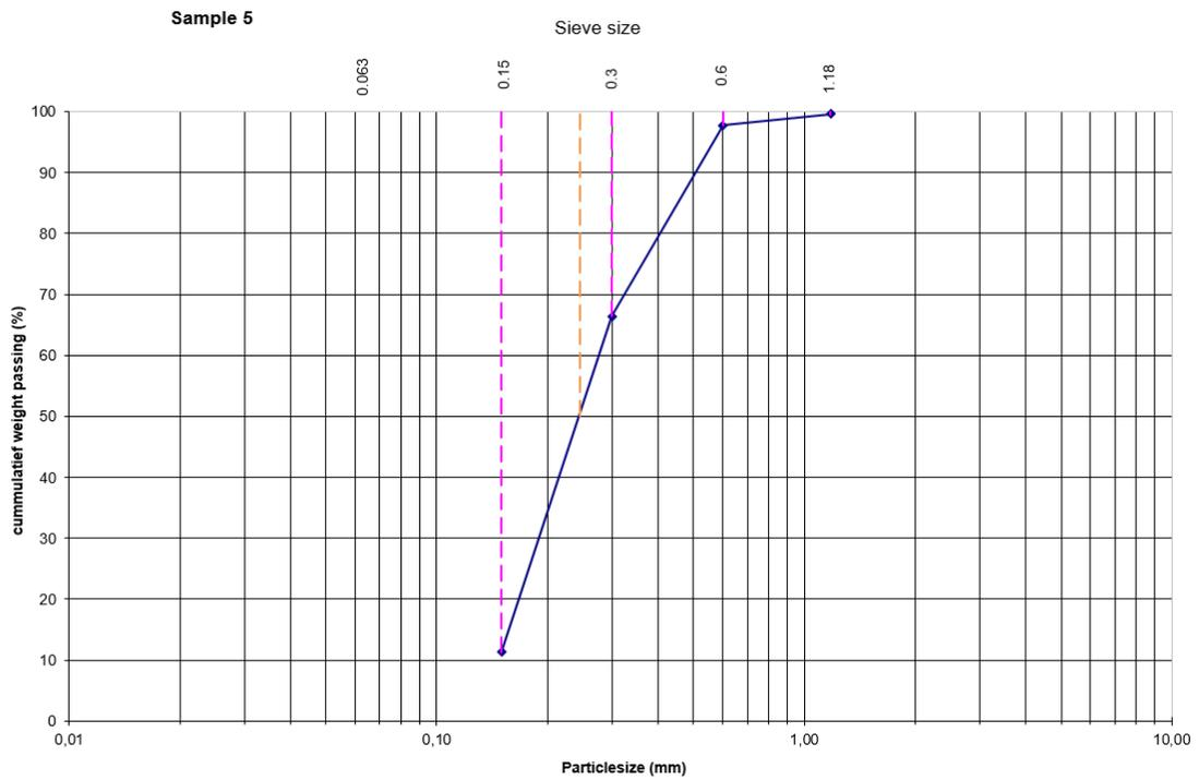
Figure A.5: Sieve curve for sediment sample 5. Indicated  $D_{50} = 0.25$  mm.
