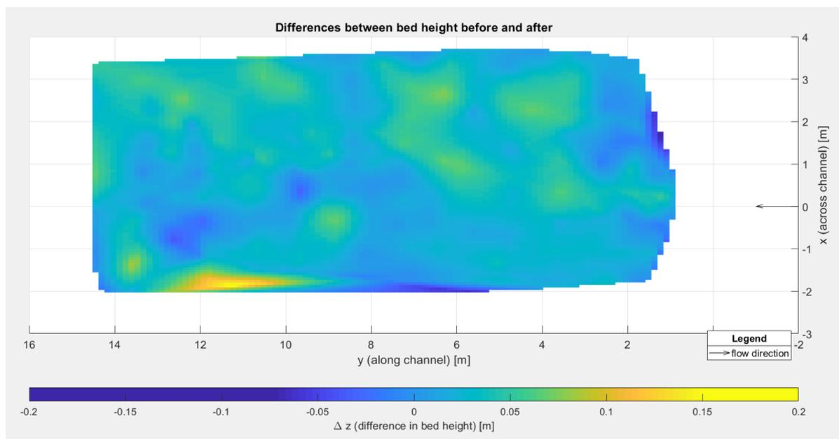
Figure B.5: Plot of the differences between the bottom profiles before and after (period 4-5)
