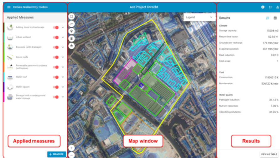
Figure 2.4: Overview of the layout of the Adaptation Support Tool of Deltares. The left panel shows the selected measures, the map in the middle presents the spatial planning and the right panel gives the results of the applied measures (source: Deltares, 2019).
