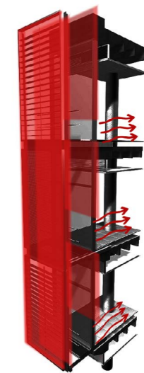
HEAT RELEASE TO THE INSIDE
