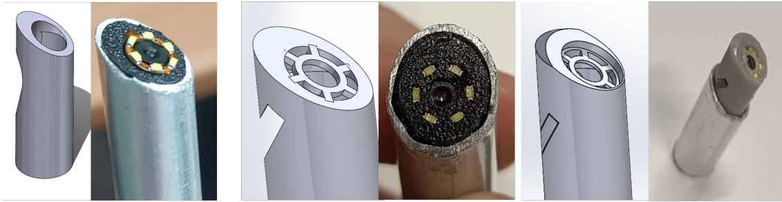
Figure 4.6: Evolution of the distal tip design: initial concept (left), second iteration with wheel structure (middle), and third iteration featuring an optical window recess (right).
