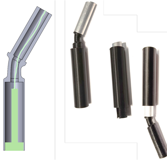
Figure 4.4: Cross-section of concept 4 with camera module in green (left) and visual explanation of movement through a trocar in three steps (right)
