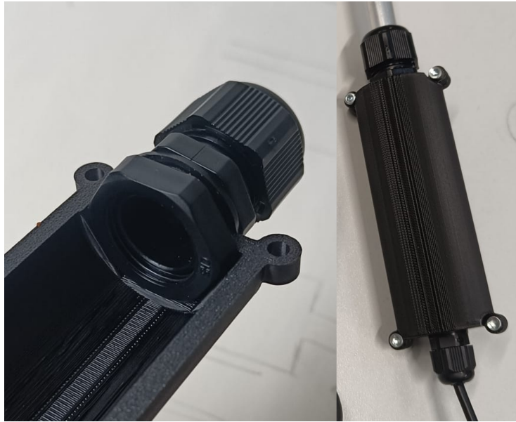
Figure 4.8: Initial longitudinal handle prototype: polymer cable gland interface (left) and bolted PLA assembly (right).
