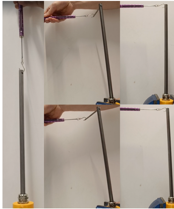
Figure 5.1: Visual Results of the Pull test (left), Torque Test (middle) and Bending test (right)
