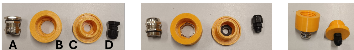
Figure 4.10: Visual representation of assembly step 1 with brass cable gland (A), top part of handle (B), bottom part of handle (C), and polymer cable gland (D).
