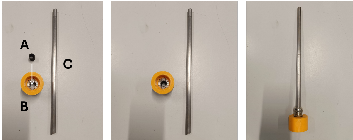
Figure 4.11: Visual representation of assembly step 2 with 3D-printed PLA spacer (A), top part of handle with brass cable gland (B), and stainless steel shaft (C).
