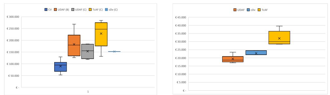
7.2.a Capital Expenditures of an OR air handling installation type A, B and C with a CV or UCV system. 7.2.b Operational expenditures of OR UCV systems, UDAF, cDV and TcAF over 10 years' time FIG. 7.2 Capital and Operational expenditures
