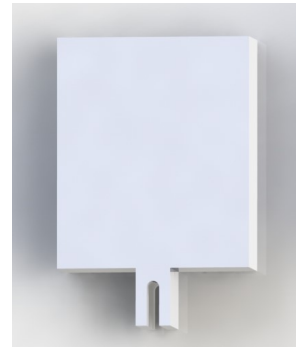
Fig. 7: Puncture-support to prevent stretching of the PDMS container when injecting the needles. It is 3D-printed with PLA. The rectangular surface is the handle and the smaller segment is positioned within the PDMS container.
