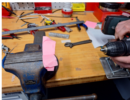
Figure B.3: The wire is twisted by clamping the wire to a bench and using the drill to twist the wire alternately in both directions. When twisting the wire, the wire is under tension, so the wire is hardened as it is pulled straight.
