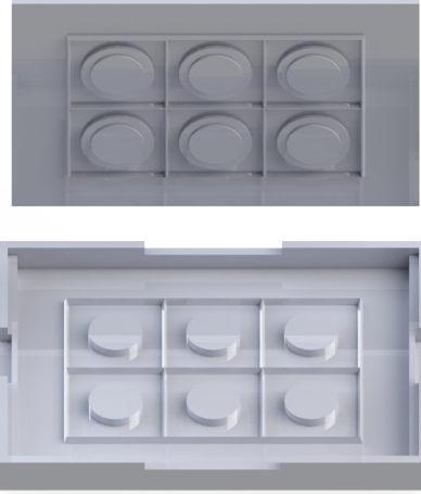
Figure 2.4: The cover is tilted, revealing the inside of the mould. On both sides of the mould, there is a circular thickening. When the lid is closed, a 1 mm gap remains between these thickenings, allowing a thin layer of PDMS to form in that space. As a result, the PDMS develops round cavities on both sides. One of these cavities, which has an edge, can be used for printing a sacrificial mould, while the lower hollow space can function as a vacuum chamber.
