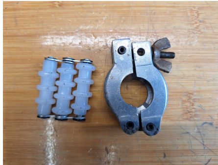
Figure B.1: A wire straightener is shown on the left and a clasper on the right. The wire straightener consists of three nylon rolling cylinders connected to each other. Some parts of the cylinders are wider, creating bumps. As the wire is pulled through the straightener, these protrusions bend the wire past its elastic point, causing plastic deformation of the wire. This occurs in several directions, resulting in the straightening of the wire.
