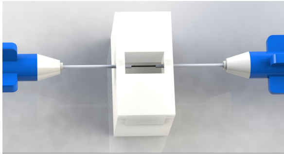
Fig. 5: Two injection needles are inserted into the PDMS container with a wire pulled through, to serve as a mould. The needles are spaced approximately 2.5 mm apart.
