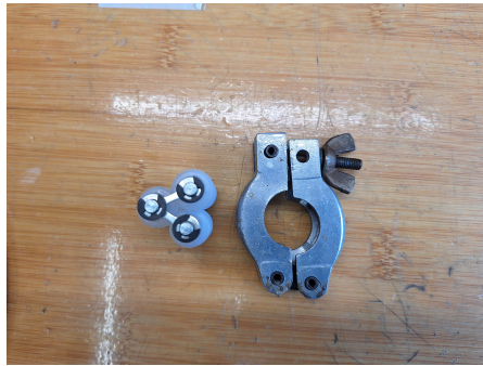
Figure B.2: A wire straightener is shown on the left and a clasper on the right. The wire straightener consists of three nylon rolling cylinders connected with each other. The rolling cylinders are clamped in the position as shown in this Figure. The wire is pulled through the centre of the three cylinders.
