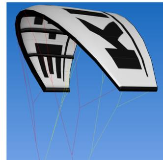
**Figure 11.23:** Visualisation kite design obtained made in SurfPlan.
