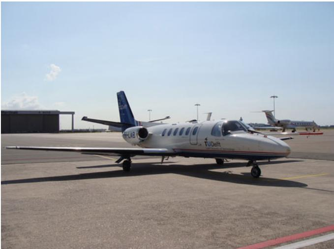
**Fig. 10.5** The PH-LAB research aircraft operated by Delft University of Technology. The Cessna Citation 550 is a CS-25 certified aircraft
