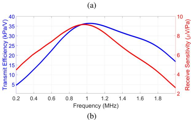
Figure 2: (a) Acoustic stack of the designed transducer array. The subdices of the PZT elements run up to 95% of the element thickness. (b) Expected performance of the designed transducer array. There are no modes with lateral vibrations within the frequency band of interest (0.2 – 2 MHz). Both the transmit efficiency and the receive sensitivity were computed at the interface between the piezo-elements and the lead.
