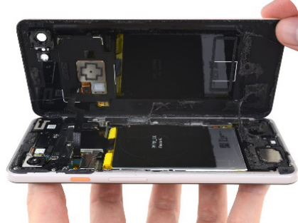
Figure 25 - Foam adhesive Pixel 3 XL (iFixit, 2018)
