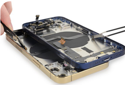
Figure 19 - Rear chassis Apple iPhone 12 Pro (iFixit, 2020)
