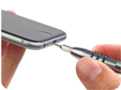
Figure 21 - Screws for display in the Apple iPhone 6 (iFixit, 2014)
