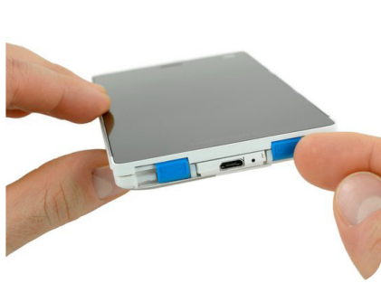
Figure 23 - Sliding clips on the Fairphone 2 (iFixit, 2015)
