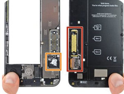
Figure 28 - Pogo Pin Connector Fairphone3 (iFixit, 2019)
