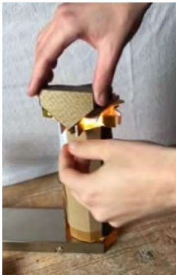
Figure 123 Closing the ring by sliding the guiding profile against the ring
