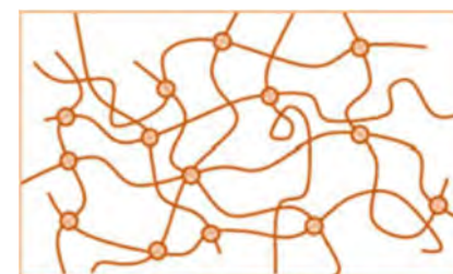
Figure 7 polymeric network of netpoints and molecular switches (Bengisu & Ferrara, 2018)
