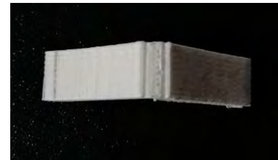
Figure 77 top view of the 45-degree sample, showing the porosity of the hinge part
