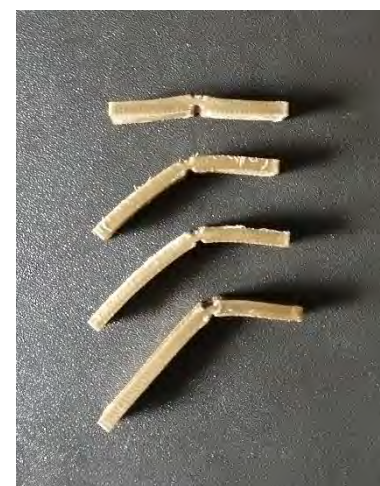
Figure 105 Recovery test samples after heating and cooling
