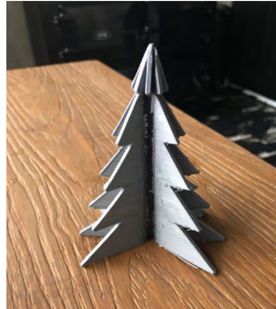
Figure 157 recovered shape showing the distance between the two unconnected sections
