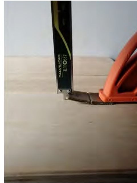
Figure 167 measuring the deformation of the samples
