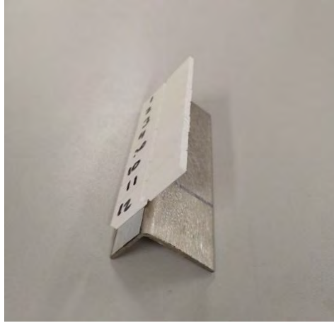
Figure 43 samples taped to an angle profile with eight at a time to ensure similar submersion time and deformation
