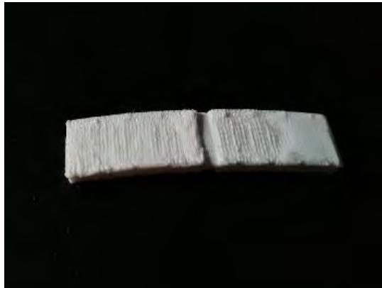
Figure 69 bottom side of a 45-degree flat sample, showing low printing quality
