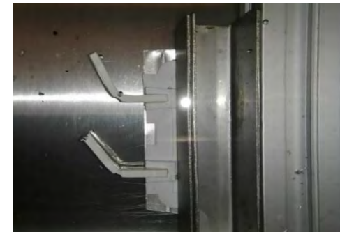
Figure 46 two samples clamped in the tool submerged in the water bath during shape recovery
