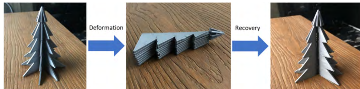
Figure 37 Christmas tree after printing (left) after deformation (middle) and after recovery (right)
