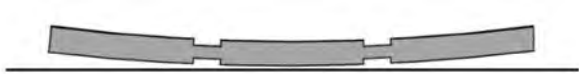
Figure 52 self-bending of the printed samples. The line beneath the sample represents the build plate. Printed samples curve upwards
