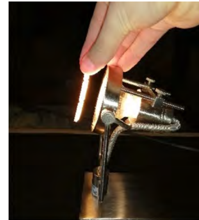
Figure 100 Test setup to test heating with a lamp
