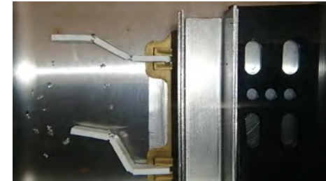
Figure 57 S shape sample recovery
