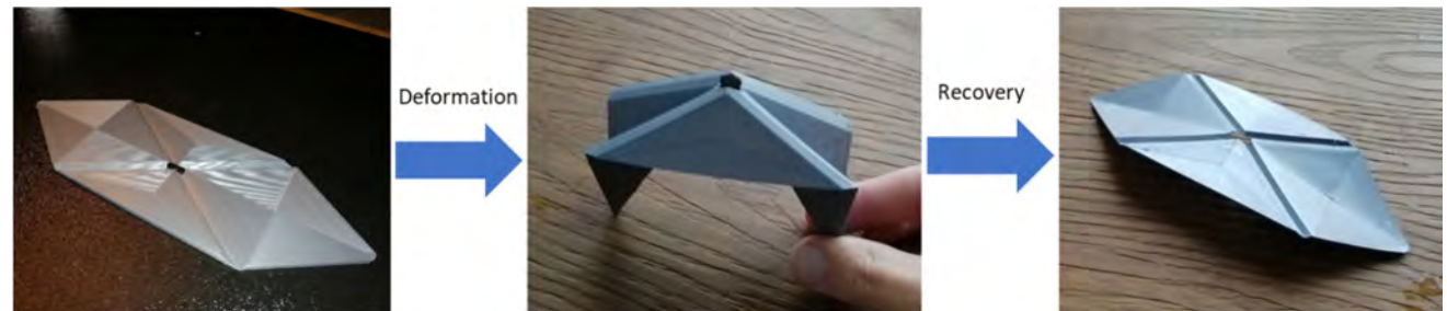
Figure 36 origami structure after printing (left) after deformation (middle) and after recovery (right)
