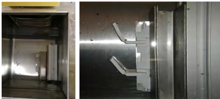
The sample holder (left) with recovering samples (right) in the water bath
