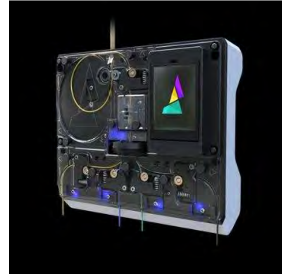
Figure 21 Mosaic Palette 2. Four different types of filament enter the device (bottom), which are then spliced and fused to create one filament wire with different properties for different sections (top) (Pires, 2020)
