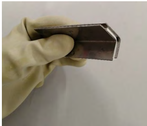
Figure 44 Samples pressed between two angle profiles to ensure similar deformation
