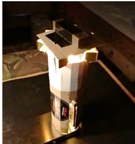
Figure 121 Test setup: A cardboard tube is placed over the lamp, and the printed ring is placed on top
