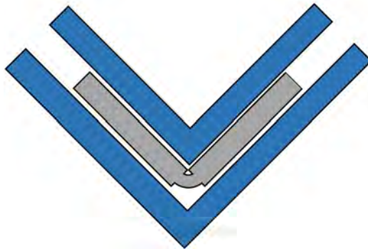
Figure 174 Bending of the sample (grey) and the bending support (blue)
