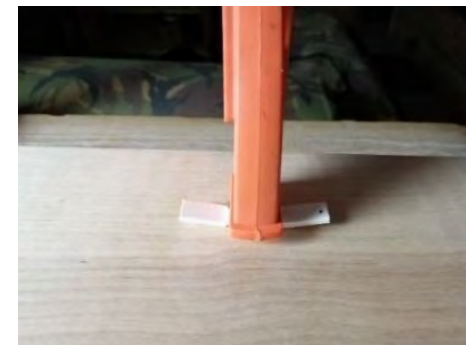
Figure 58 clamping method for measuring deformation after recovery
