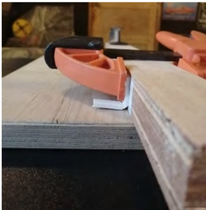
Figure 74 clamping of the samples that recovered more than 100% and measuring of the remaining deformation
