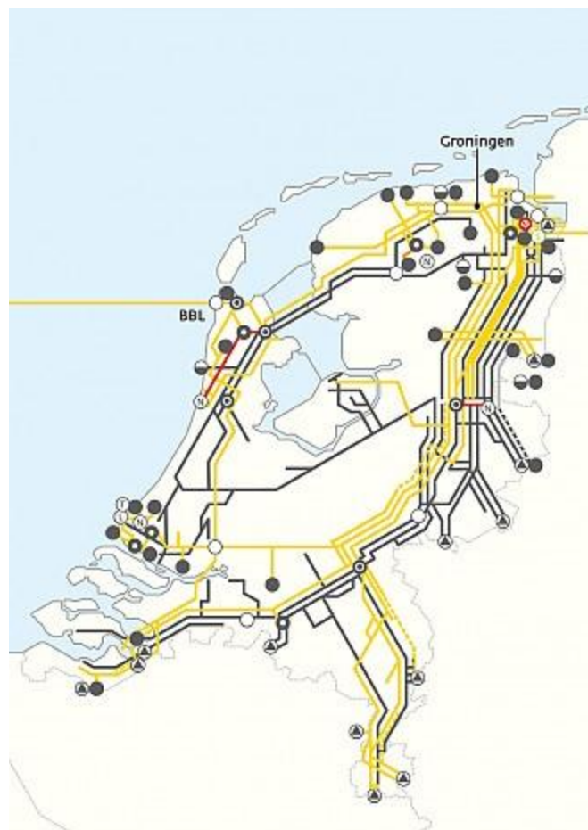
Figure 4.1: The Dutch transmission network (Gasunie, 2013b)
