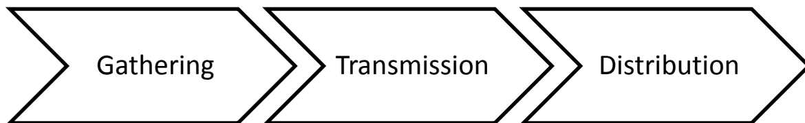
Figure 4.4: Types of Pipelines in the Gas system (Based on: (Prieto et al., 2012))
