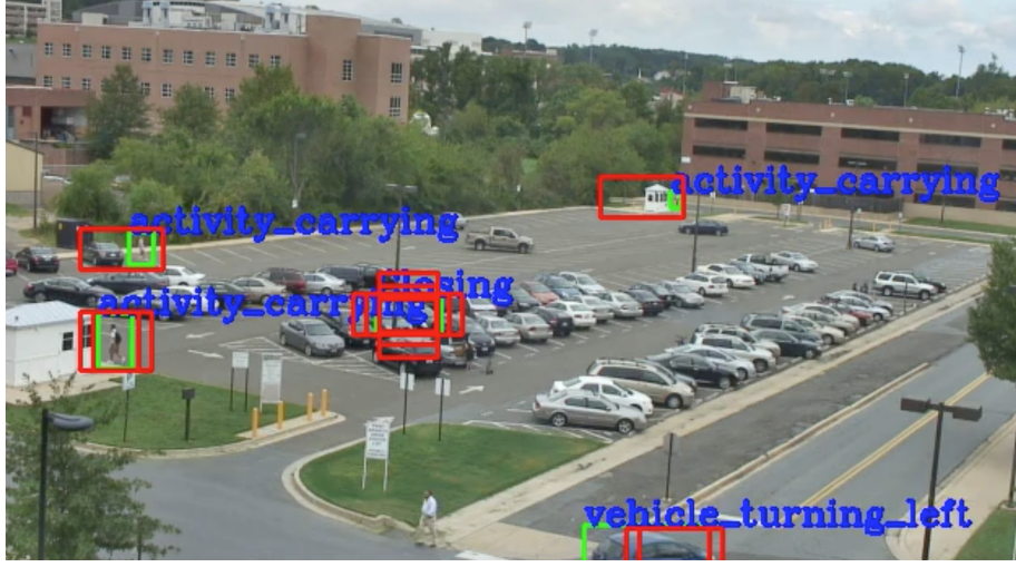
Figure 3-4: Anchor cuboid matching. The anchor cuboids (red) are matched to the ground-truth tubelet (green). For this, the spatio-temporal IoU is used as a criterion.
