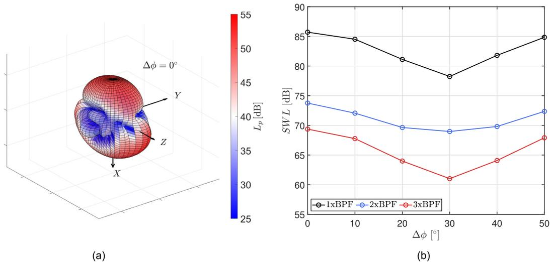
FIG. 14. (a) Three-dimensional  $L_p$  directivity of the first BPF harmonic tone for the DP case with  $\Delta\phi = 0^\circ$ . (b) SWL trends for the tones at the first, second, and third BPF harmonics for different phase angles. For both images, the acoustic interference effects are accounted for by including the contributions of the three propellers.
