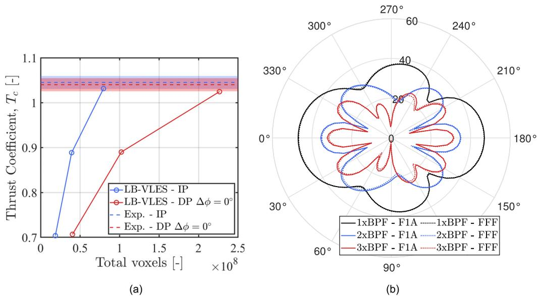
FIG. 5. (a) Evolution of the thrust coefficient against the total number of voxels for the IP (blue) and the central propeller of the  $\Delta\phi = 0^\circ$  configuration (red). The experimental results for each case are shown as dashed lines, with uncertainty represented by shaded regions. (b) Comparison between LB/F1A and LB/FFF noise directivity results.  $L_p$  emitted by the central propeller of the DP configuration at  $\Delta\phi = 0^\circ$  at a distance of  $100D$ .
