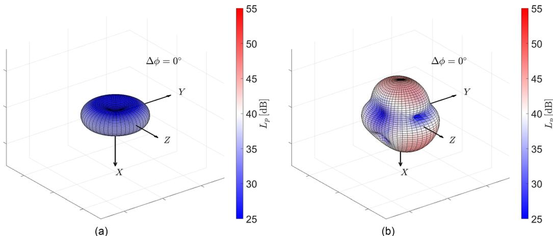
FIG. 10. Three-dimensional  $L_p$  directivity of the first BPF harmonic tone for the DP case with  $\Delta\phi = 0^\circ$ . Only the contribution of the central propeller is accounted for. (a) Considering the steady loading contribution and (b) considering the unsteady loading contribution.
