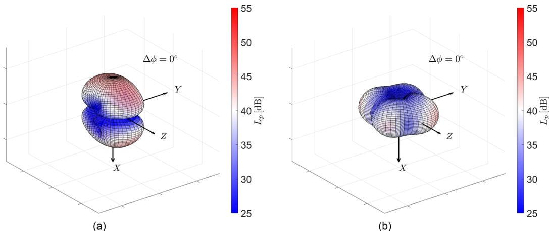
FIG. 11. Three-dimensional  $L_p$  directivity of the first BPF harmonic tone for the DP case with  $\Delta\phi = 0^\circ$ . Only the contribution of the central propeller is accounted for. (a) Considering the axial loading contribution and (b) considering the tangential loading contribution.
