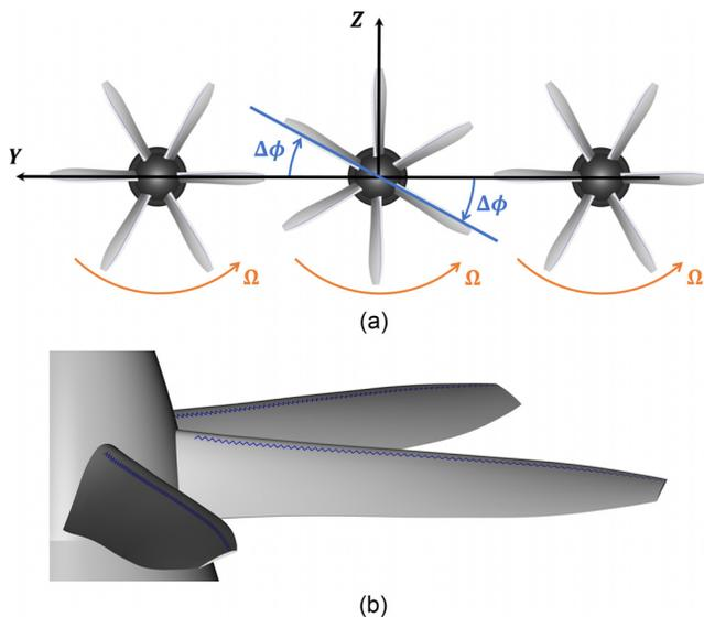
FIG. 3. (a) Front view of the array of propellers defining the global reference frame, angular velocity  $\Omega$ , and relative phase angle  $\Delta\phi$ . (b) Close-up on the zig-zag tripping applied on the blades.
