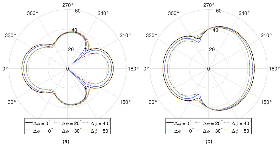
FIG. 13. Far-field sound  $L_p$  directivity comparing the distributed central propeller cases for different phase angles. The first BPF harmonic tone is depicted. Microphones distributed in the XY (a) and XZ (b) planes, respectively.
