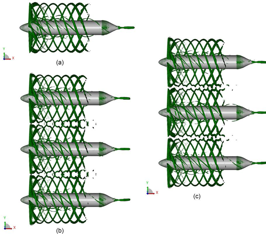
FIG. 6. Isosurface computed through the  $\lambda_2$  criterion with a value of  $\lambda_2 = -2 \times 10^6 \text{ 1/s}^2$ : isolated-propeller case (a), distributed-propeller case with  $\Delta\phi = 0^\circ$  (b), distributed-propeller case with  $\Delta\phi = 30^\circ$  (c).
