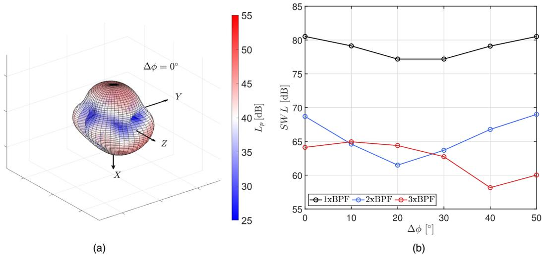
FIG. 12. Noise directivity of the DP central propeller contribution. (a) Three-dimensional  $L_p$  directivity of the first BPF harmonic tone for the DP case with  $\Delta\phi = 0^\circ$ . (b) SWL trends for the tones at the first, second, and third BPF harmonics for different phase angles.
