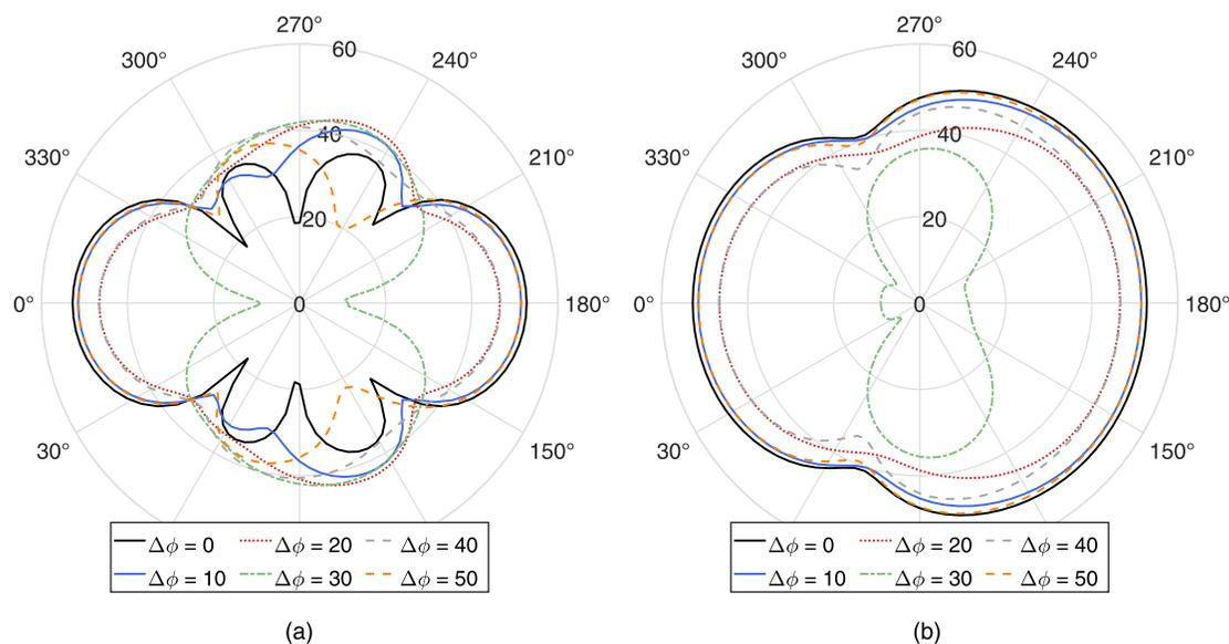
FIG. 15. Far-field sound  $L_p$  directivity comparing the DP cases varying  $\Delta\phi$ . The first BPF harmonic tone is depicted. The acoustic interference effects are accounted for by including the contributions of the three propellers. Microphones distributed in the XY (a) and XZ (b) planes, respectively.
