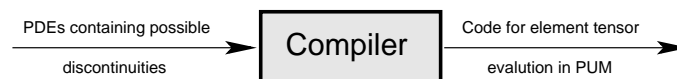
Figure 4.1 Input/output of the PUM compiler. The compiler receives the variational formulations in the UFL syntax as input and generates automatically required C++ code compatible with UFC.
