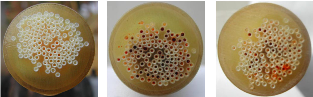
Figure 2 - Photos of the concentrate side of a membrane, left photo: new membrane; middle photo: membrane after back flushing; right photo: membrane after chemical cleaning. Clearly the blocked capillaries are visible.
