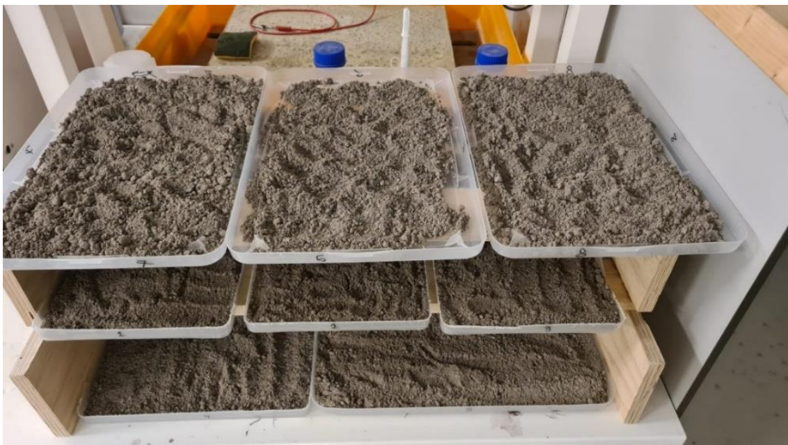
Figure 4.3: Setup for large-scale carbonation of BFA1, displaying plastic trays for extensive carbonation.
