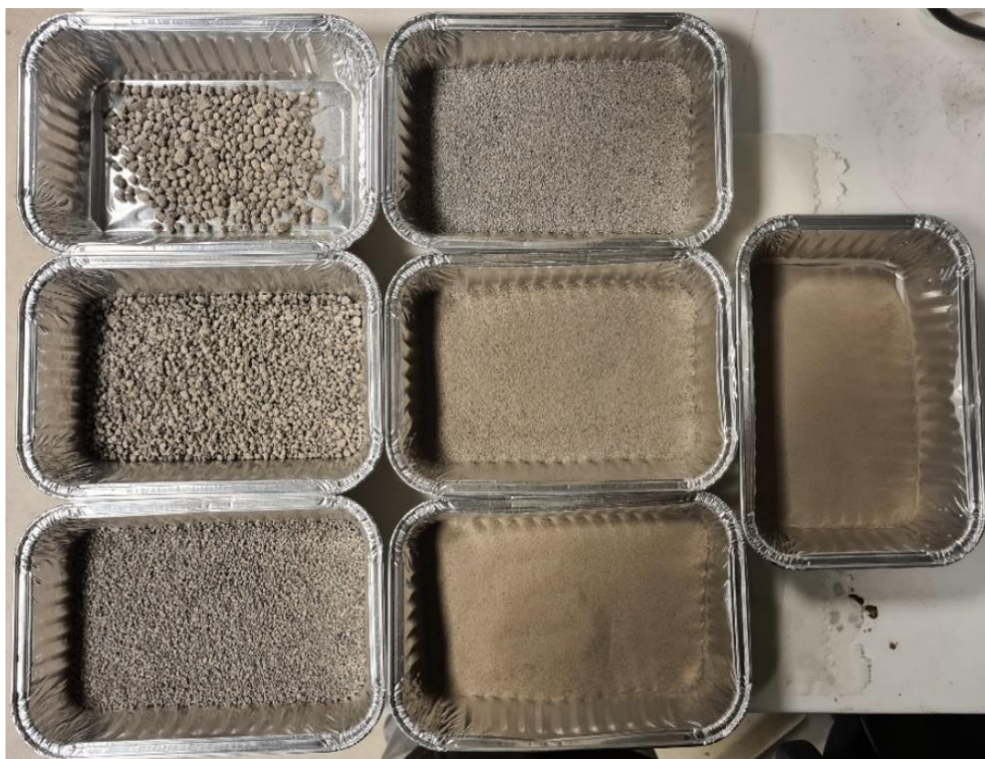
Figure 4.9 : Visual representation of the different particle size fractions of carbonated biomass fly ash (BFA-H-C) obtained through sieve analysis.
