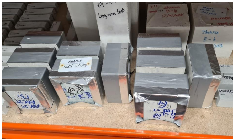
Figure 5.4: Concrete samples prepared and sealed for freeze-thaw testing.
