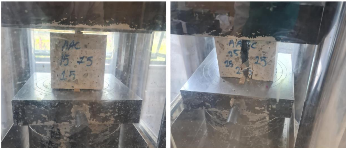
Figure 5.3: Setup of the tensile strength test for a concrete cube specimen.
