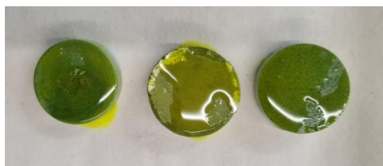
Figure 6.2: Samples impregnated with epoxy in preparation for the SEM-EDX test.
