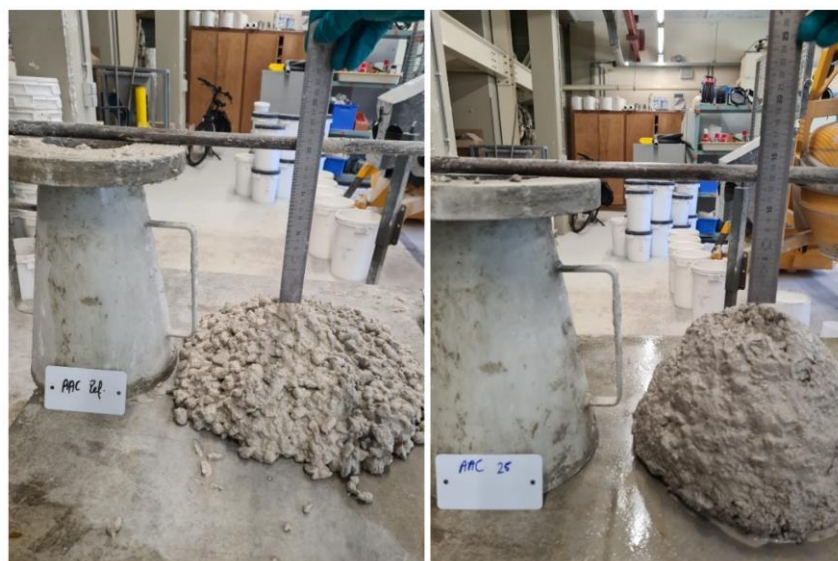
Figure 5.1: Slump test for reference concrete (left) and concrete incorporating 25% BFA1 (right), illustrating the workability differences due to ash incorporation.
