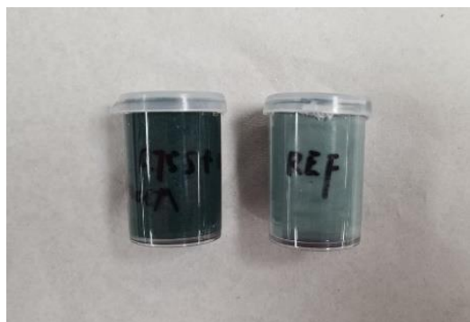
Figure 6.1: Paste samples for microstructural analysis, with 'Paste-BFA' on the left incorporating biomass fly ash and 'Paste-REF' on the right consisting only of slag.
