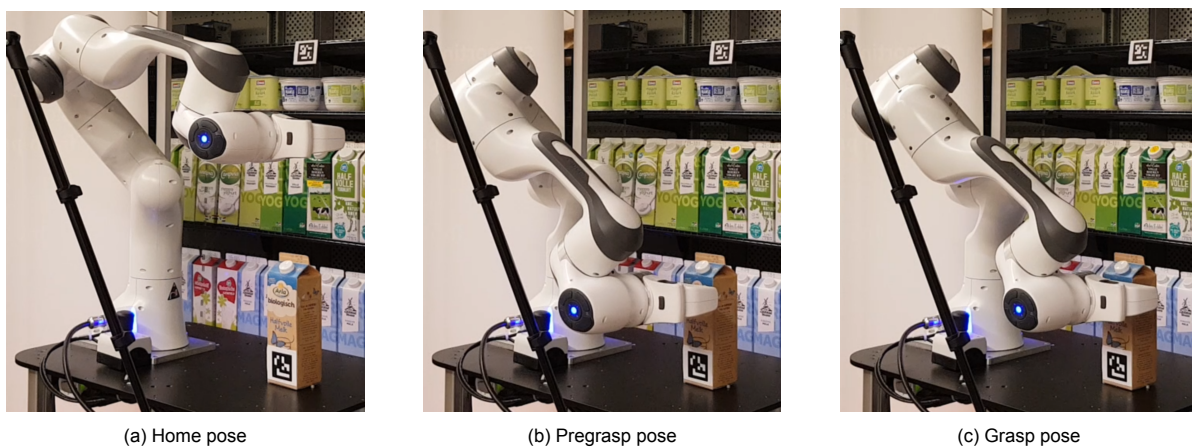
Figure 4.5: Predefined joint space poses for grasping an object from the supply.
