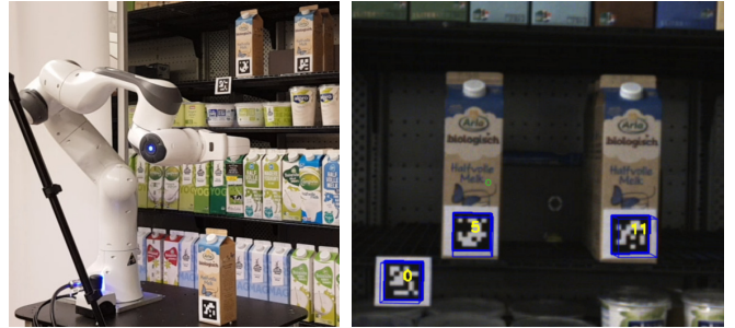
Fig. 1: Impression of SyRePOE stocking a shelf. On the left the Franka Emika Panda, the objects and shelves are shown. On the right the view of the shelf for pose detection is visible.
