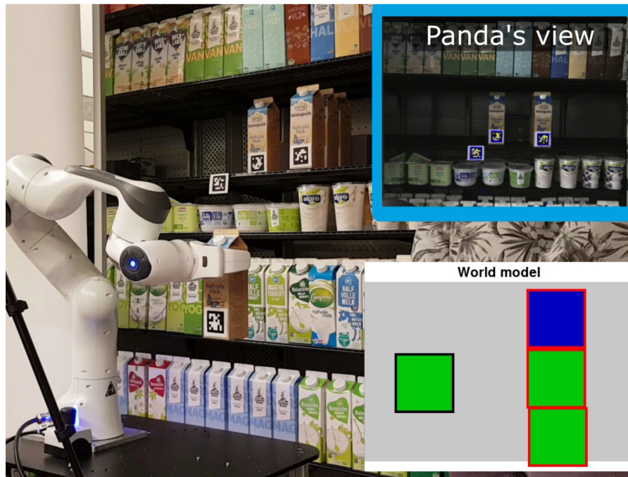
Figure 4.4: Impression image of SyRePOE stocking a shelf. On the left the Franka Emika Panda can be seen, together with objects and shelf marked with Aruco markers. On the top right the view of the shelf used for pose detection is visible. On the bottom right a visualisation of the world model is shown.
