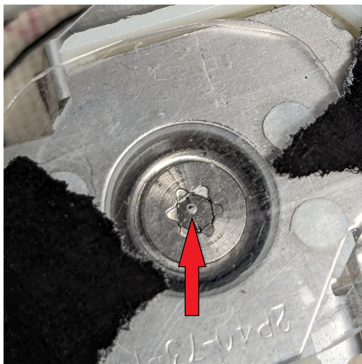
Figure 3.6: The ^{241}\text{Am} source of the smoke detector with a plastic single-hole collimator (0.5mm), which is indicated with the red arrow.
