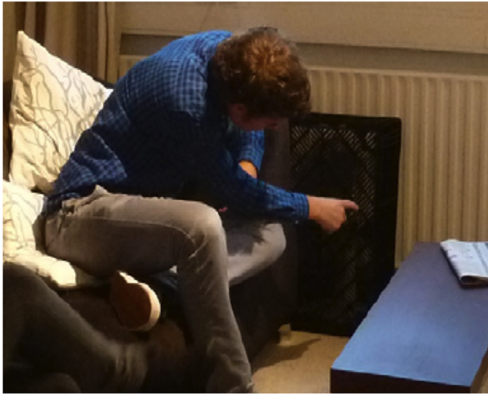
Fig. 9. Air inlet simulated with a fan hidden in a crate.
