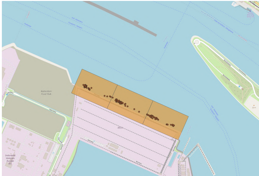
Figure G.2: The polygons used to determine berth 1(right) to berth 3 (left) for EECV, Rotterdam. With the average position of all vessels that visited the terminal in 2024.
