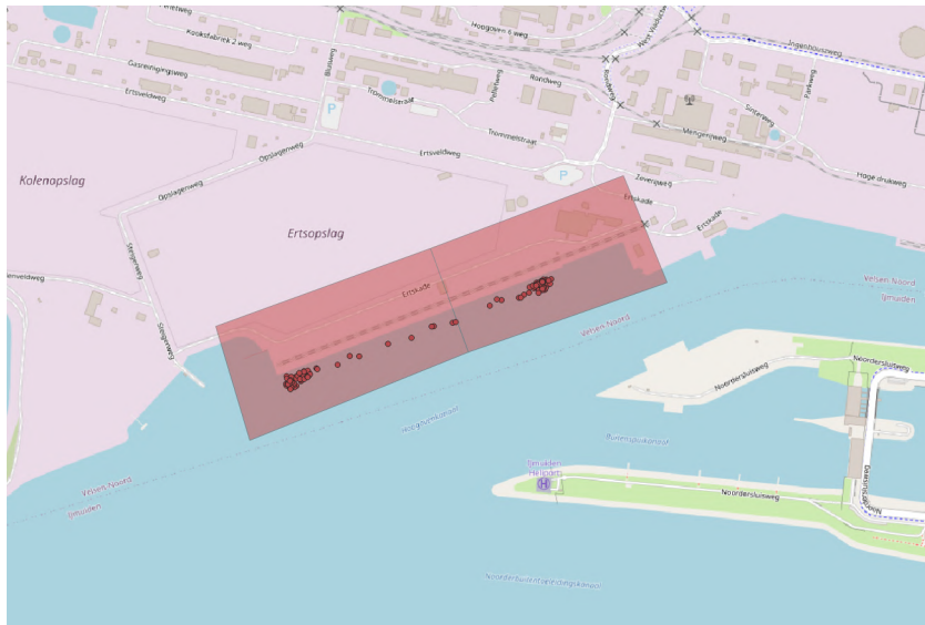
Figure G.3: The polygons used to determine berth 1(left) and berth 2(right) for Tata Steel IJmuiden. With the average position of all vessels that visited the terminal in 2024.
