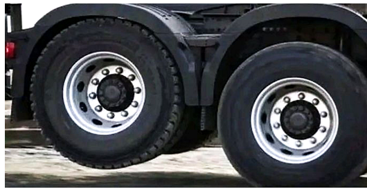
Figure 10: The floating wheel of a truck – as a well-known example of structurally enacted situated behavior.
